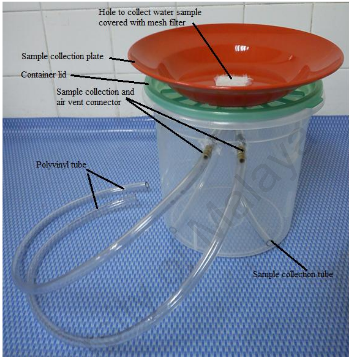
Plate 3.5: Soil water sampler
