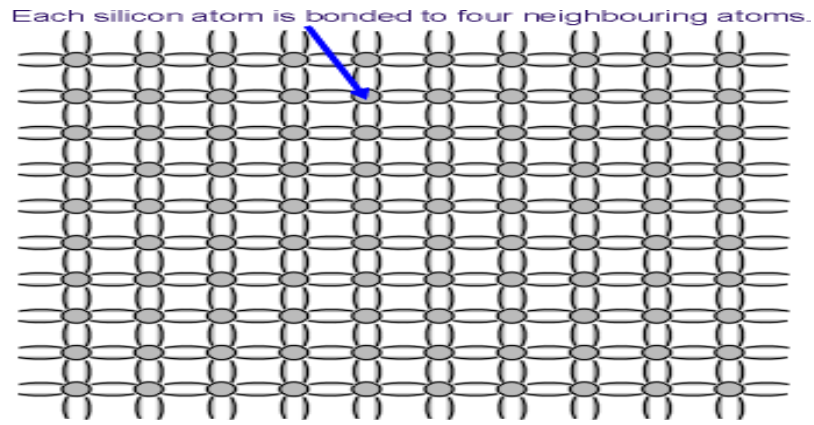
Figure 2.10: Regular atomic structure of a monocrystalline solar cell (PVEO, 2013b)
