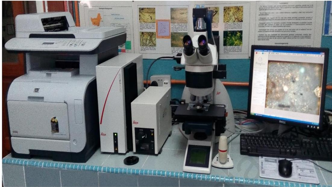
**Figure 3.9: LEICA CTR DM6000 Orthoplan Microscope used in this study**
