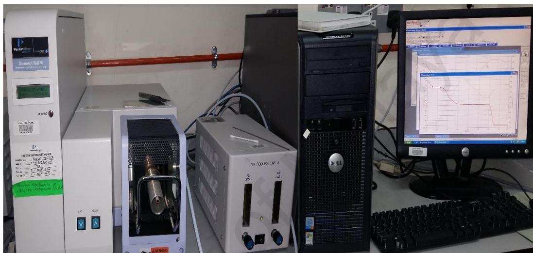
**Figure 3.7: Perkin Elmer Diamond Thermogravimetric-Differential Thermal Analyser (TG-DTA) used in this study**
