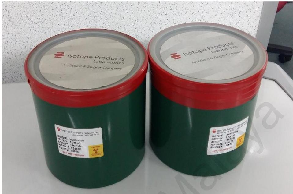
**Figure 3.5: Standard gamma-ray calibration source**
