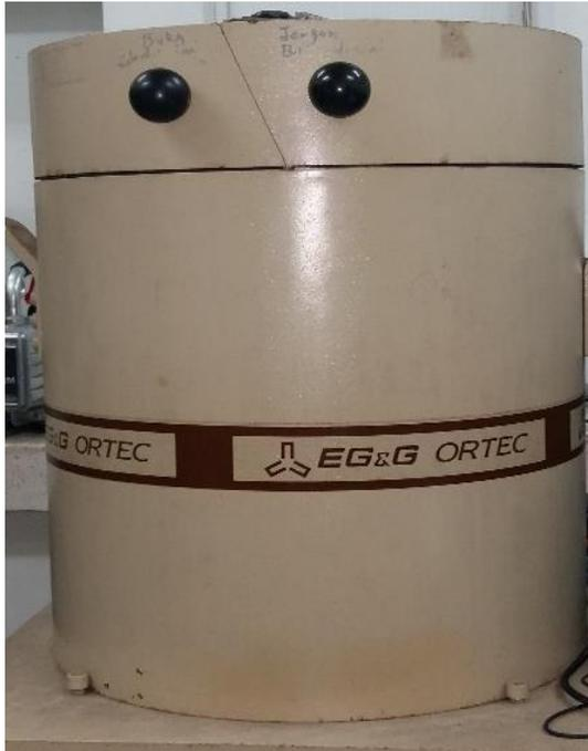
(a) Lead shielded HPGe detector
