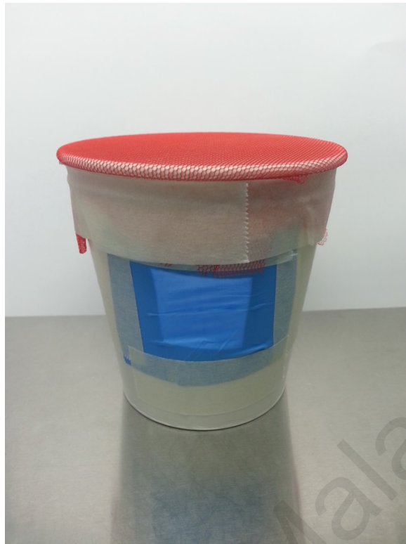
Figure 3.2: Mosquito cup covered with netting and window tightly covered with glove pieces
