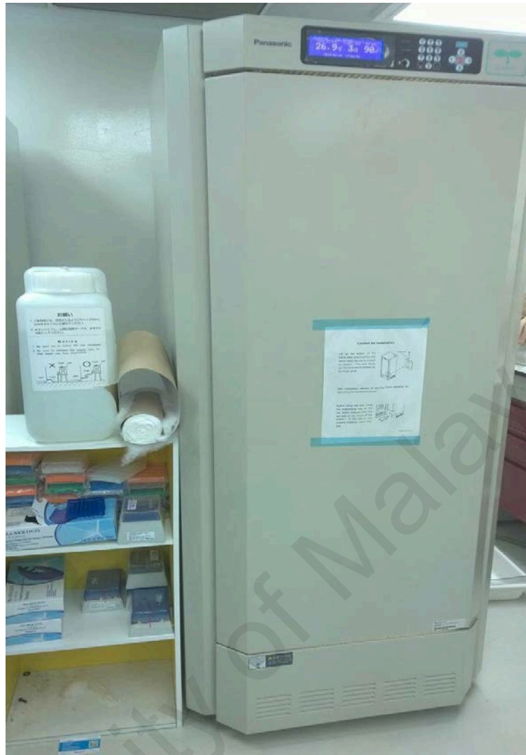
Figure 3.6: Growth chamber with regulated temperature and humidity; 12 hL 12H D
