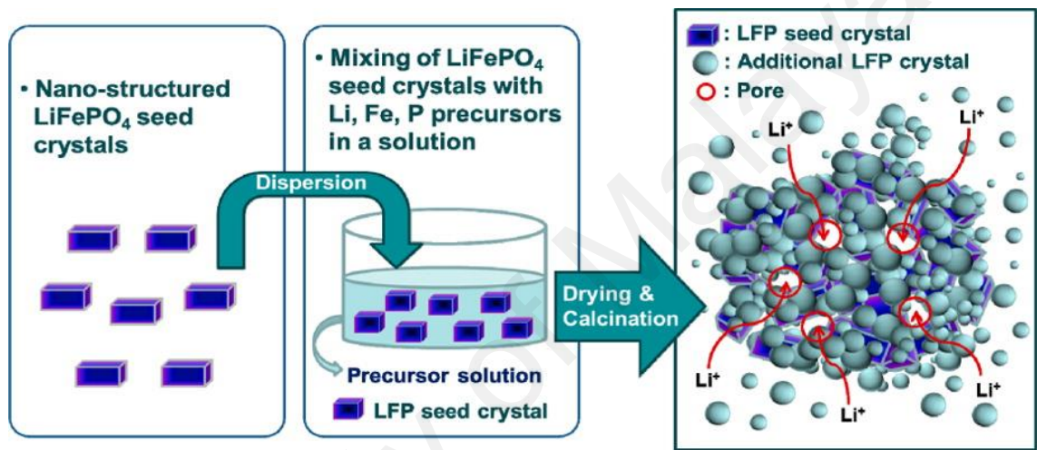
Figure 2.14: Nanoscale \text{LiFePO}_4 crystals as seed crystals for second crystallization process (Han et al., 2013)
