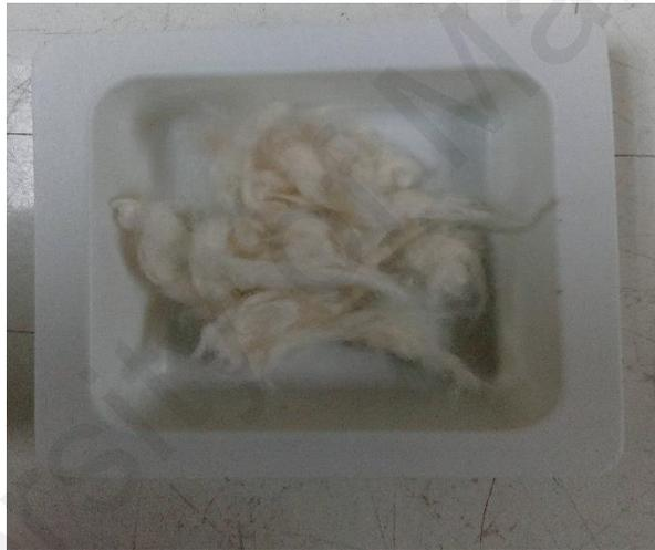
Figure 3.2: The dried silk fibers after treated with  $\text{CaCl}_2$  and dried for 24 hours
