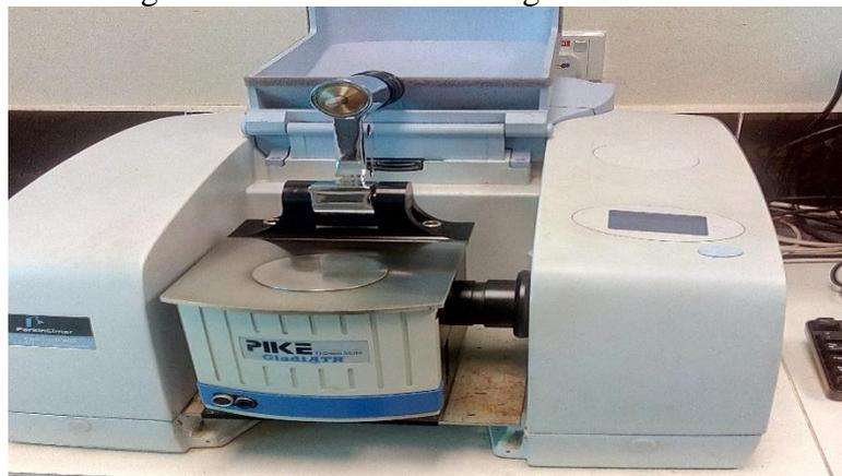
Figure 3.7: Fourier Transform Infrared Spectroscopy (FTIR)
