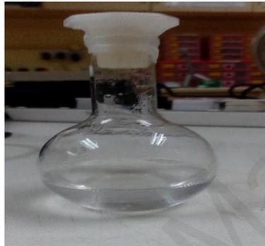
Figure 3.4: The mixture of small cut fibers with PVA solution
