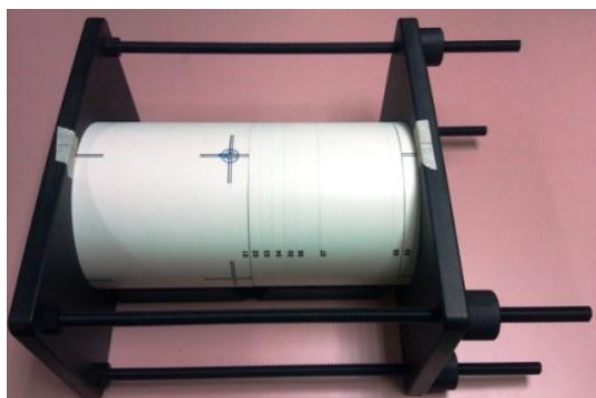
Figure 3.6: The cylindrical IMRT head and neck phantom (model 002HN, CIRS)
