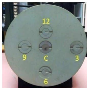
Figure 6.2: Photograph showing the IMRT head and neck phantom with the inserts for the OSLD adaptors. The positions of the adaptors were labeled with respect to the center (C) adaptor
