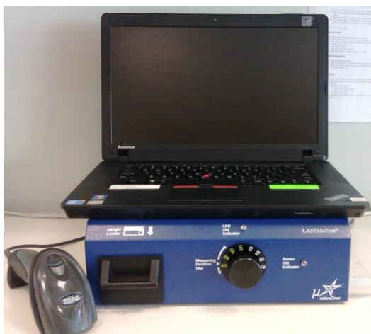
Figure 3.11: The MicroStar reader system which consists of a loader, a barcode scanner and a laptop
