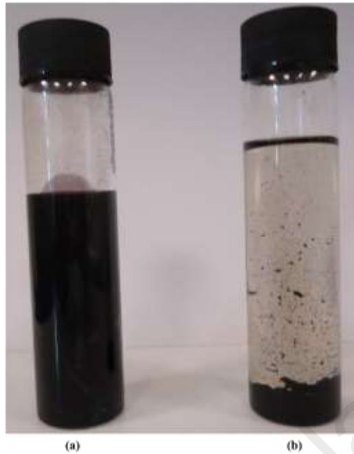
Figure 5.1: Photograph of (a) DBSA-doped PNVC-Ppy/GO dispersed in DMF; (b) PNVC-Ppy/GO (without DBSA) dispersed in DMF
