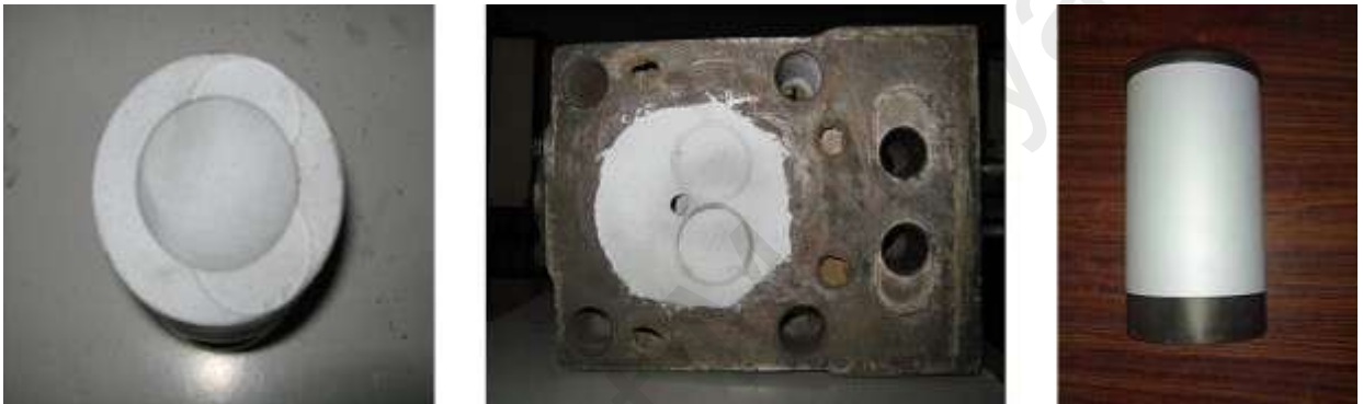
Figure 2.9: Photographic view of piston, cylinder head and cylinder liner after coating (Rajendra et al., 2010)
