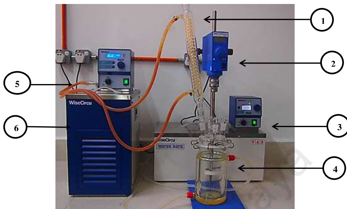
Figure 3.4: Experimental set up used to perform biodiesel production. (1) reflux condenser; (2) overhead mechanical stirrer; (3) circulating water bath; (4) Jacketed glass batch tank reactor (1 l); (5) hoses; (6) Refrigerator.
