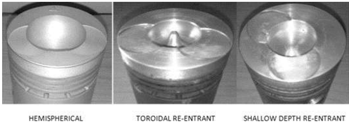
Figure 2.7: Photographic view of different combustion chambers employed (Jaichandar & Annamalai, 2012)
