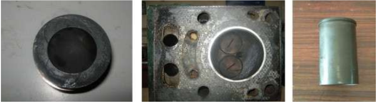
Figure 2.8: Photographic view of piston, cylinder head and cylinder liner before coating (Rajendra et al., 2010)
