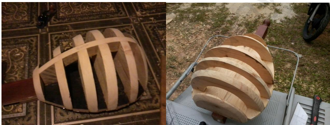
Figure 4.7: Body mould for gambus
