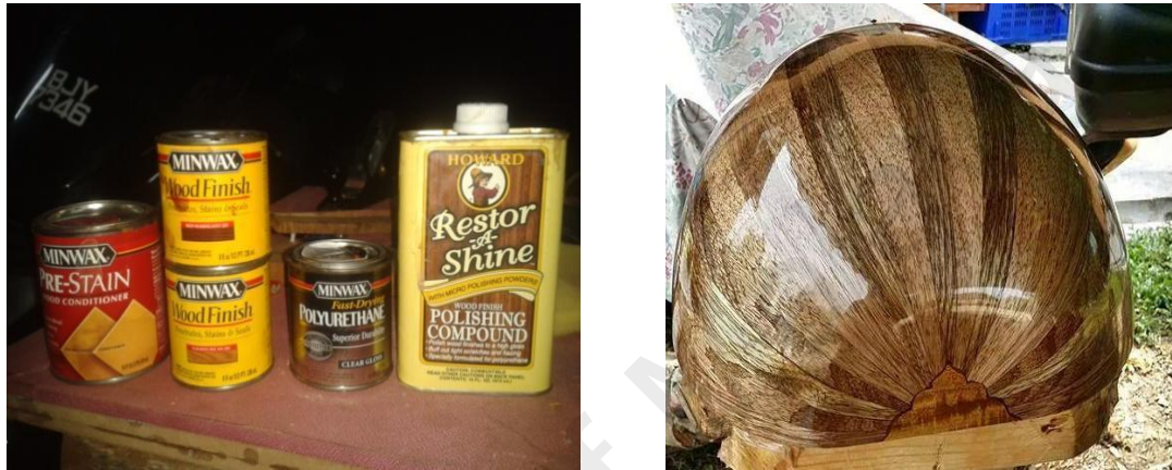
Figure 4.12: Finishing materials and polished bowl-back result
