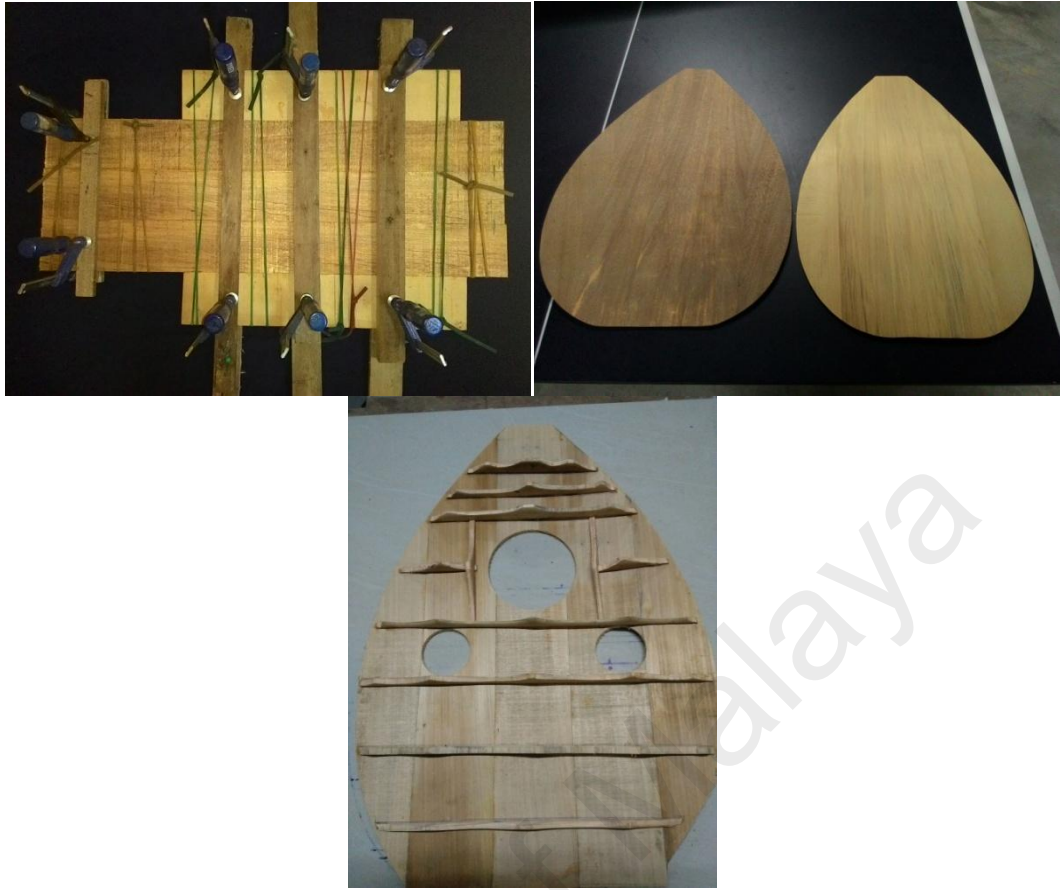
Figure 4.10: Soundboard making process
