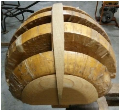
Figure 4.8: First strip glued to tampuk dalam
