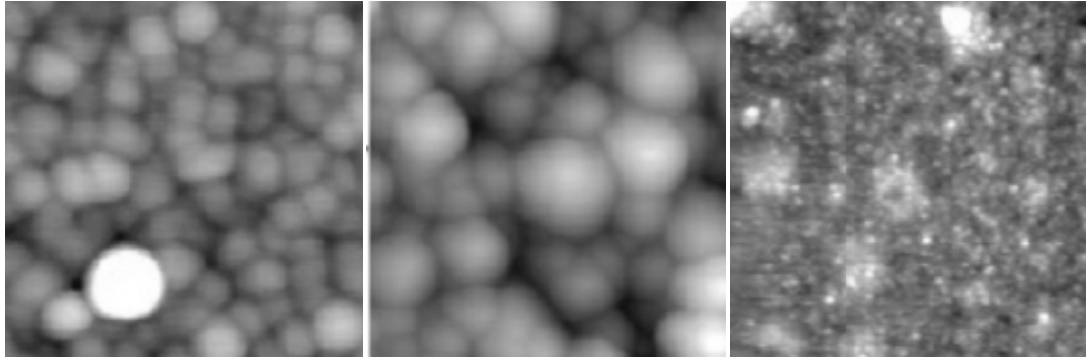
Figure 2.20: The AFM study of structurally disordered Ag(Sn)I thin films (Mohan & Sunandana, 2013).
