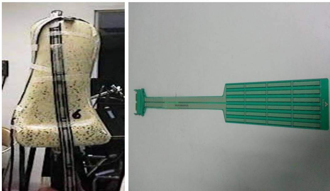
Figure 2.45: (left) Rincoe and (right) F-socket force-sensing resistors are made to be paper-thin and pliable to allow easy insertion between the socket and residual limb (reproduced from (Polliack et al., 1998) and Tekscan(2007))
