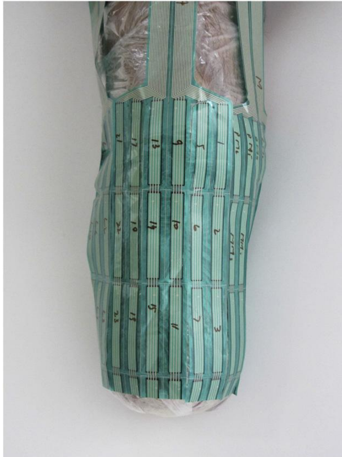
Figure 4.1: Placement of sensors on a residual limb
