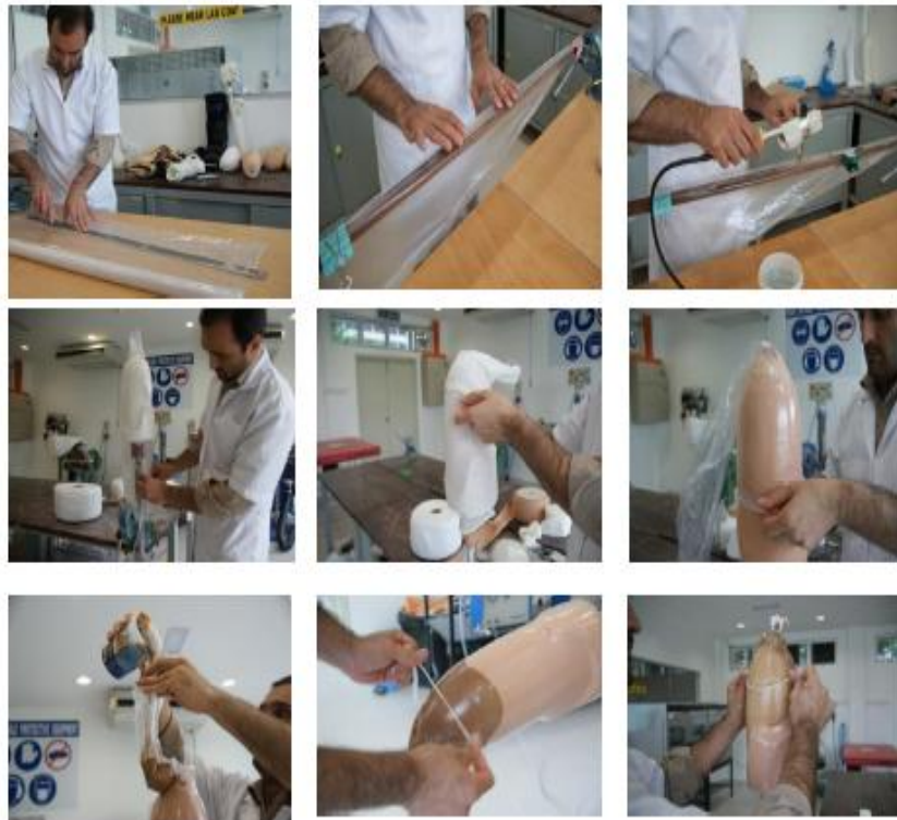
Figure 2.32: Procedures for making a definitive prosthesis
