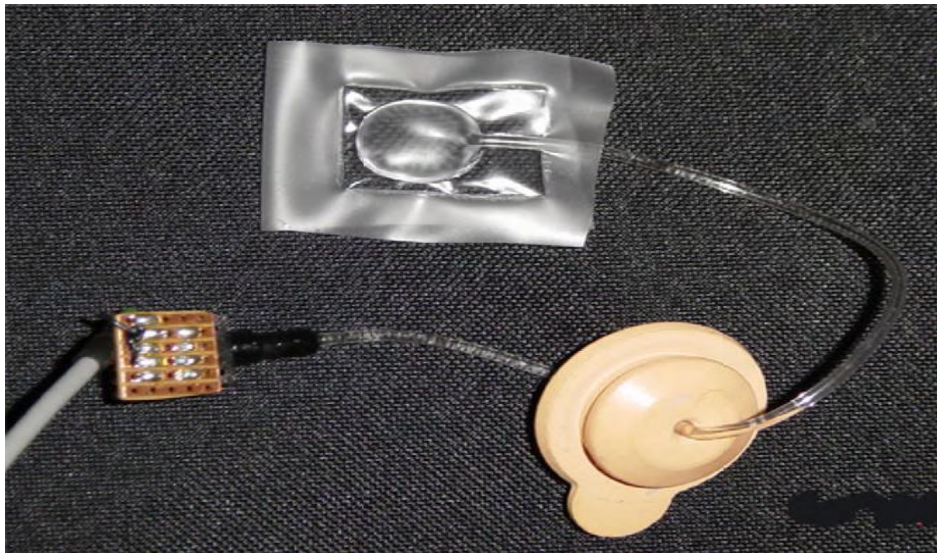
Figure 2.43: Electrohydraulic pressure transducers (Abu Osman et al., 2010).
