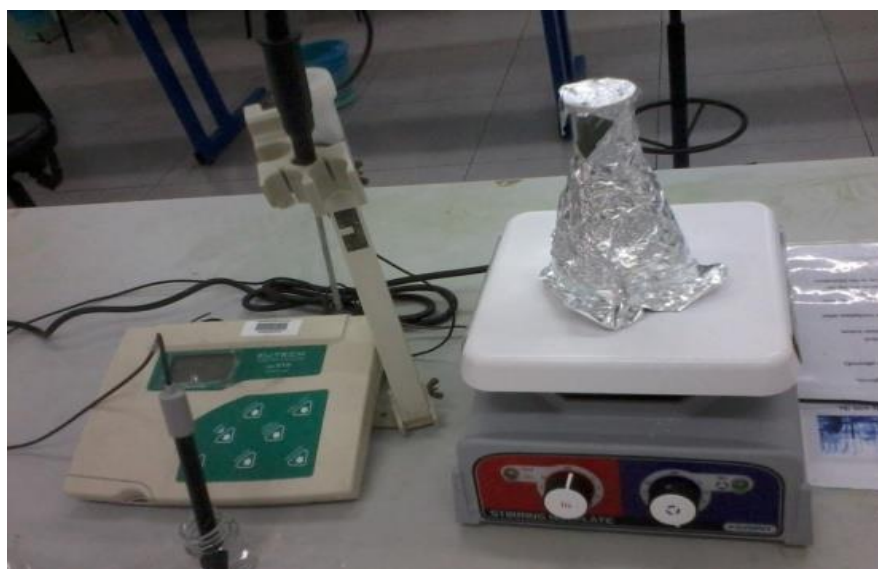
Plate 3.1 Aluminum foil wrapped conical flask due to the high photo sensitivity index of metal oxalate ligands
