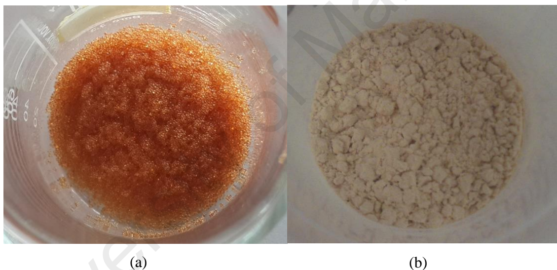
Figure 3.2: The Amberlite resin (a) beads (620 – 830 µm) and (b) powder (20 – 40 µm) following size reduction.
