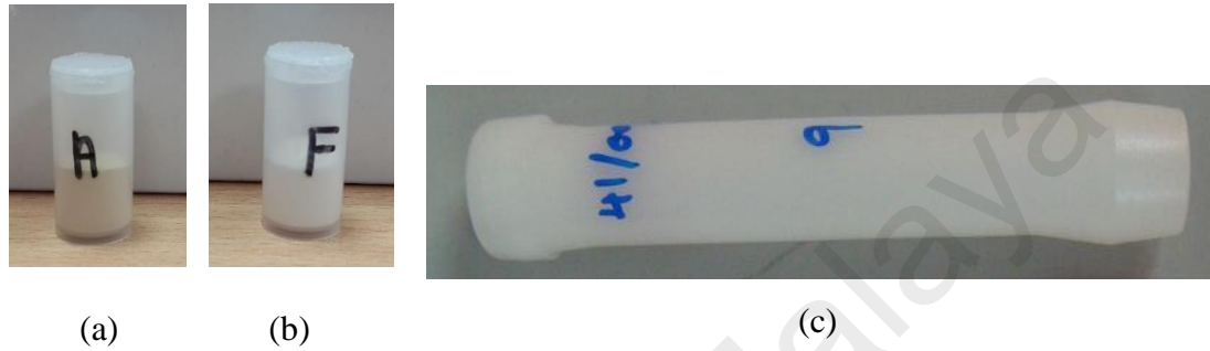
Figure 3.5: The microparticles; (a) ^{152}\text{Sm} -Amberlite and (b) ^{152}\text{Sm} -Fractogel, were sealed in individual polyethylene vial and placed into separate (c) polyethylene ampoule for neutron activation.
