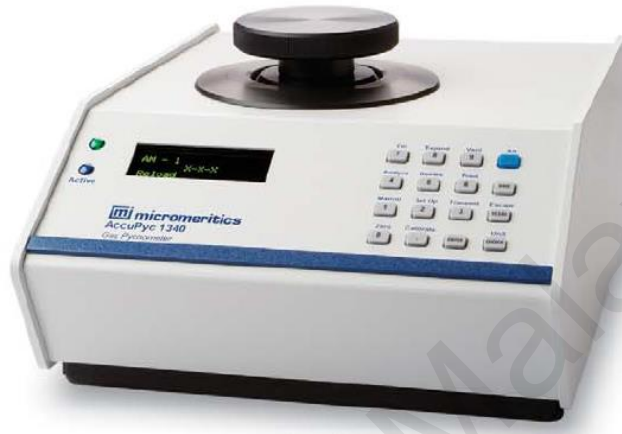
Figure 4.3: Helium gas pycnometer (AccuPyc II 1340, Micromeritics Ins. Corp., Georgia, USA)
