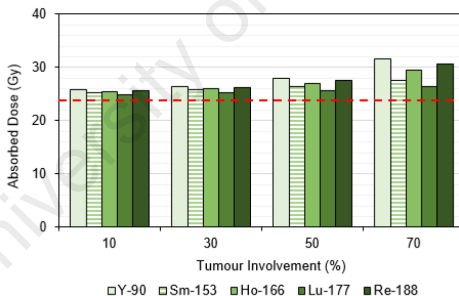
Figure 7.1: Absorbed dose to normal liver for all radionuclides and tumour involvements (for 10 % lung shunting (LS) and tumour-to-normal liver uptake ratio (T/N) of 5), when 120 Gy is delivered to the tumour. Red dotted line indicated the normal liver dose of 24 Gy as estimated by the partition model (PM).
