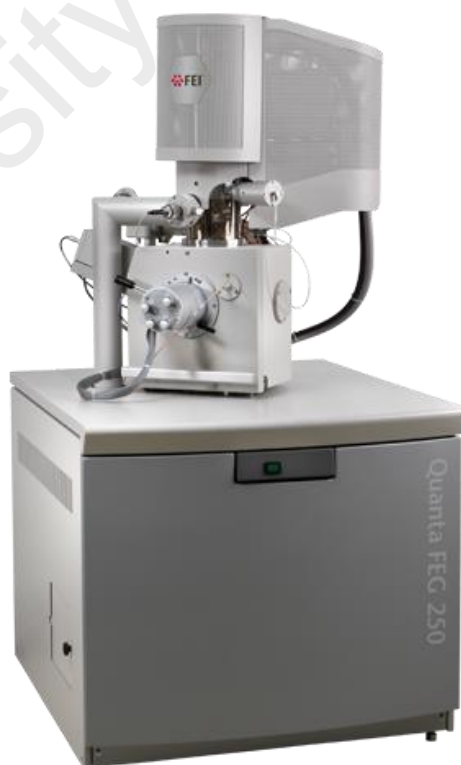
Figure 4.2: The field emission scanning electron microscope (FESEM) system (Quanta FEG 250, FEI, Oregon, USA).
