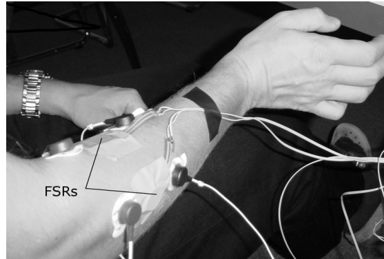
Figure 2.2: Placement of FSRs on the surface of subject's arm. (Adapted from Amft et al., 2006).
