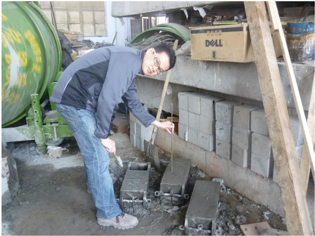
Figure 4.16: Preparation of concrete test cubes.
