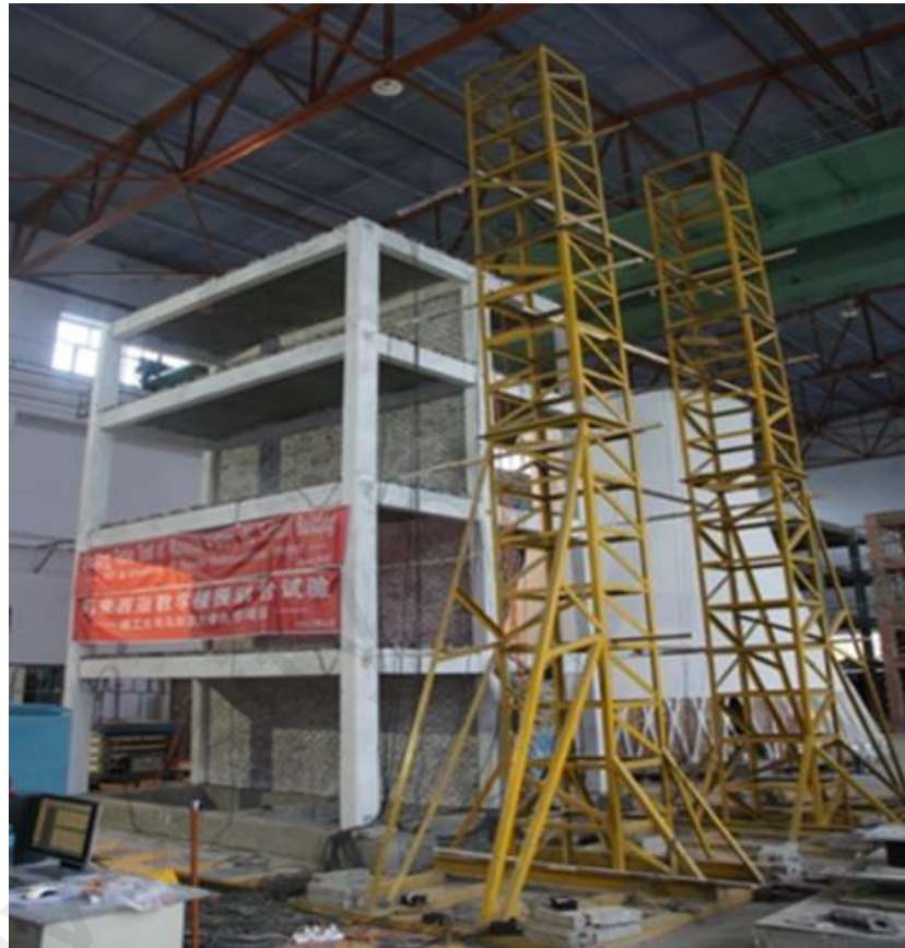
Figure 4.1: Scaled model on 5mx5m shake table.
