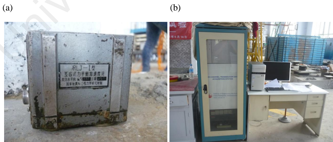
Figure 4.2: Instrumentation: (a) accelerometer and (b) data recorder.
