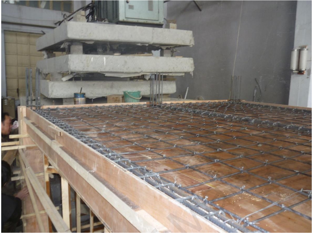
Figure 4.14: Slab and beam reinforcement.
