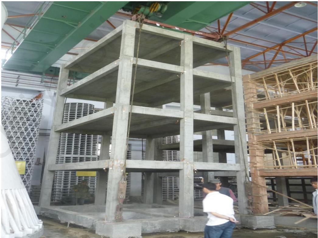
Figure 4.19: Transporting the scaled model to the shake table.
