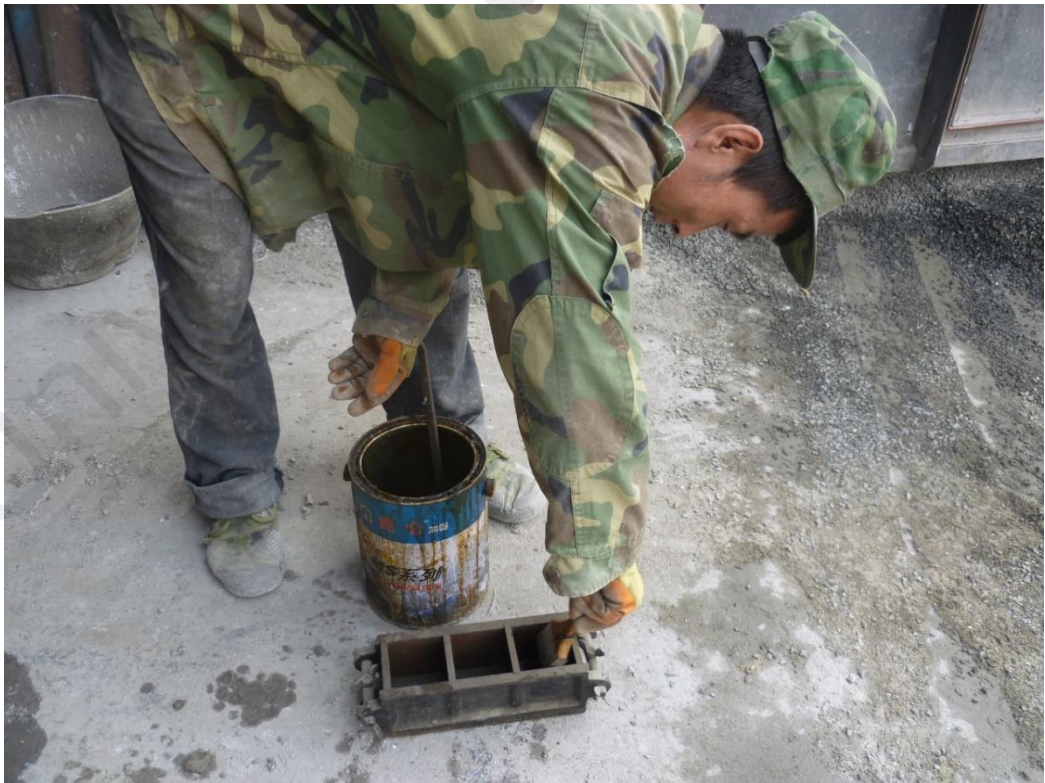
Figure 4.21: Preparation of mortar test cubes.
