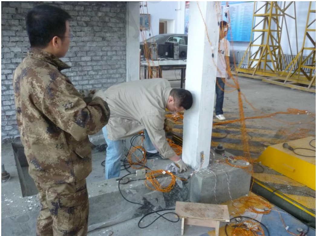
Figure 4.5: Installation of accelerometers.
