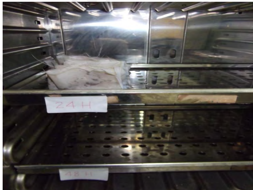
Plate 3.17 Nylon Bag Dried in Oven After Washed
