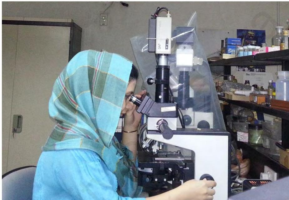
**Figure 3.3: Digitizing the monogenean specimens, using Leica digital camera DFC 320 attached to Leica DMRB microscope.**
