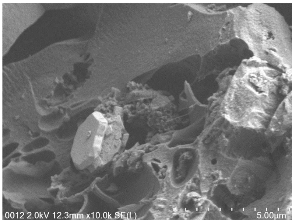
**Figure 4.8:** FESEM image of SDBS-doped polypyrrole/activated carbon (PPy/SDBS/AC) composite.
