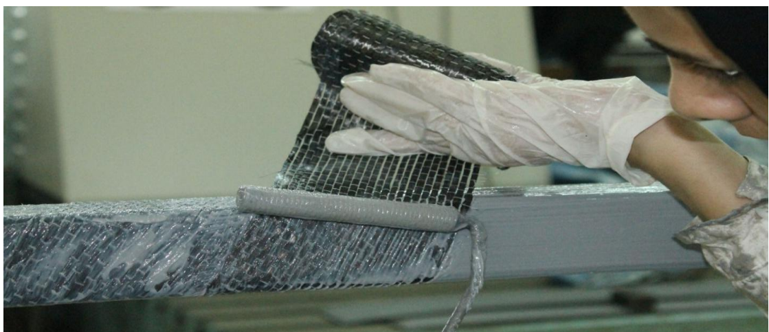
Figure 3.8 Applying CFRP wrap on the surface of the SHS
