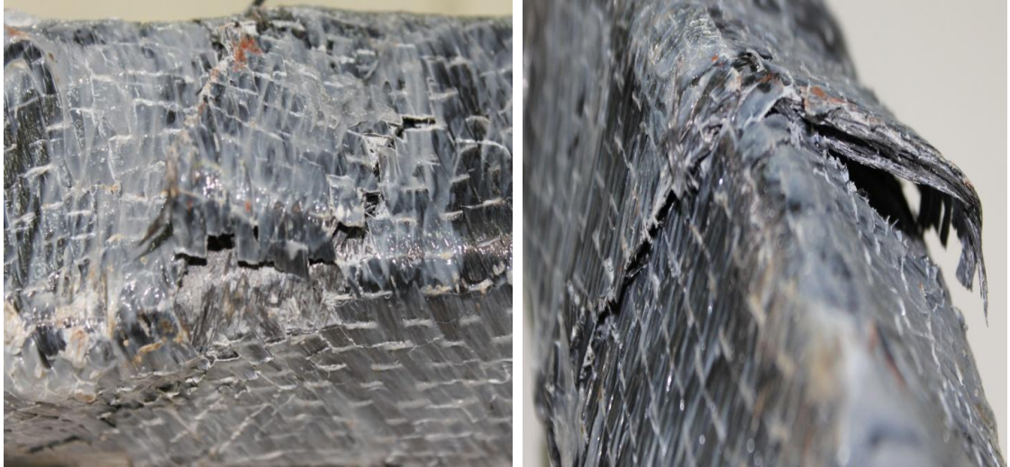
Figure 4.26 CFRP rupture and debonding failure mode of SHS1 RRRS60°
