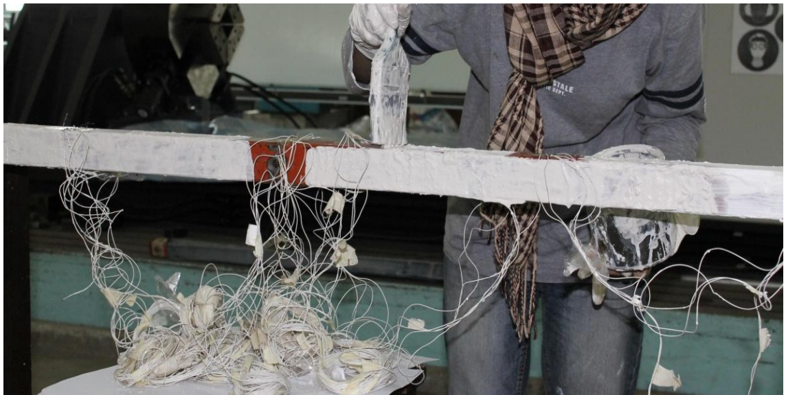
Figure 3.13 Control beams painted with a lime wash
