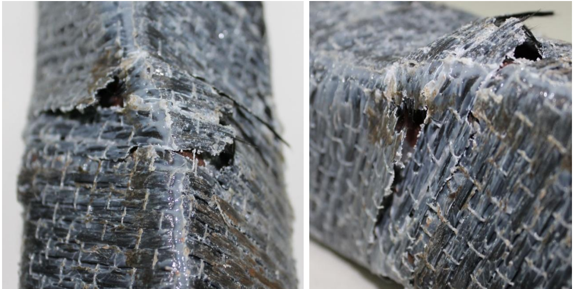
Figure 4.20 CFRP rupture and debonding failure modes of SHS1 R60°
