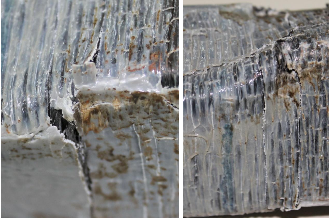
Figure B.1 CFRP splitting failure mode of SHS1 v90°
