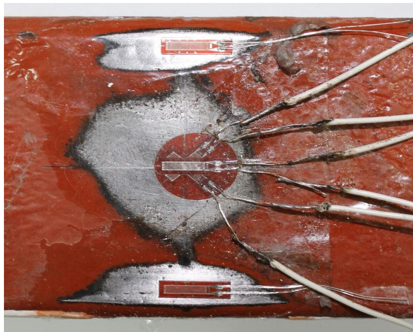
Figure 3.16 Strain gauge arrangement pattern on the control beam on side 1
