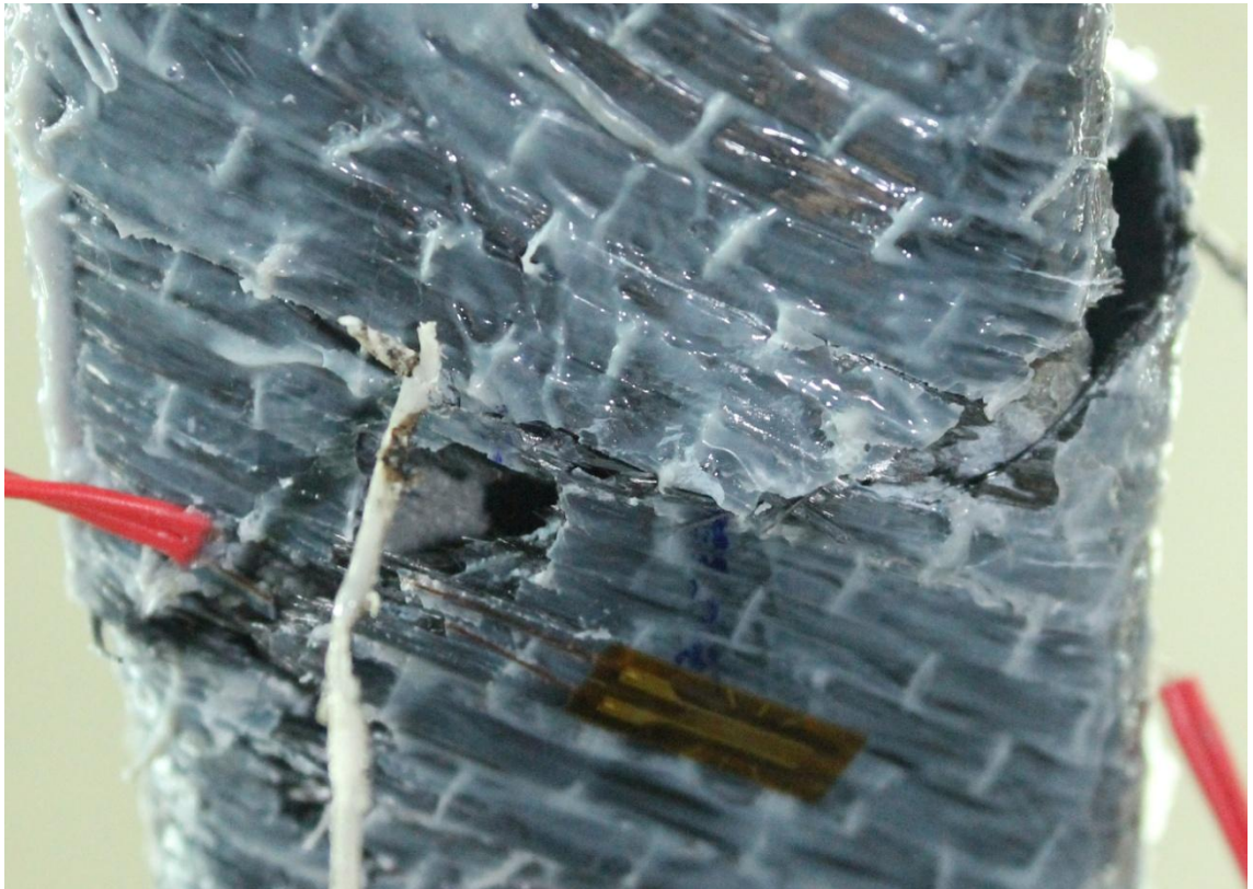
Figure 4.25 CFRP rupture and debonding failure mode of SHS1 RSR60°
