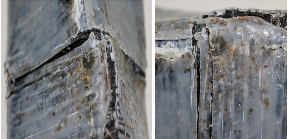
Figure 4.19 CFRP splitting failure mode of SHS1 V90°
