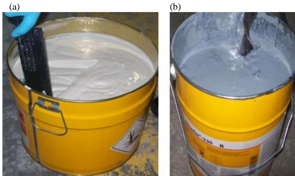
Figure 3.4 Sikadur ®-330, (a) component A (resin), (b) component B (hardener)
