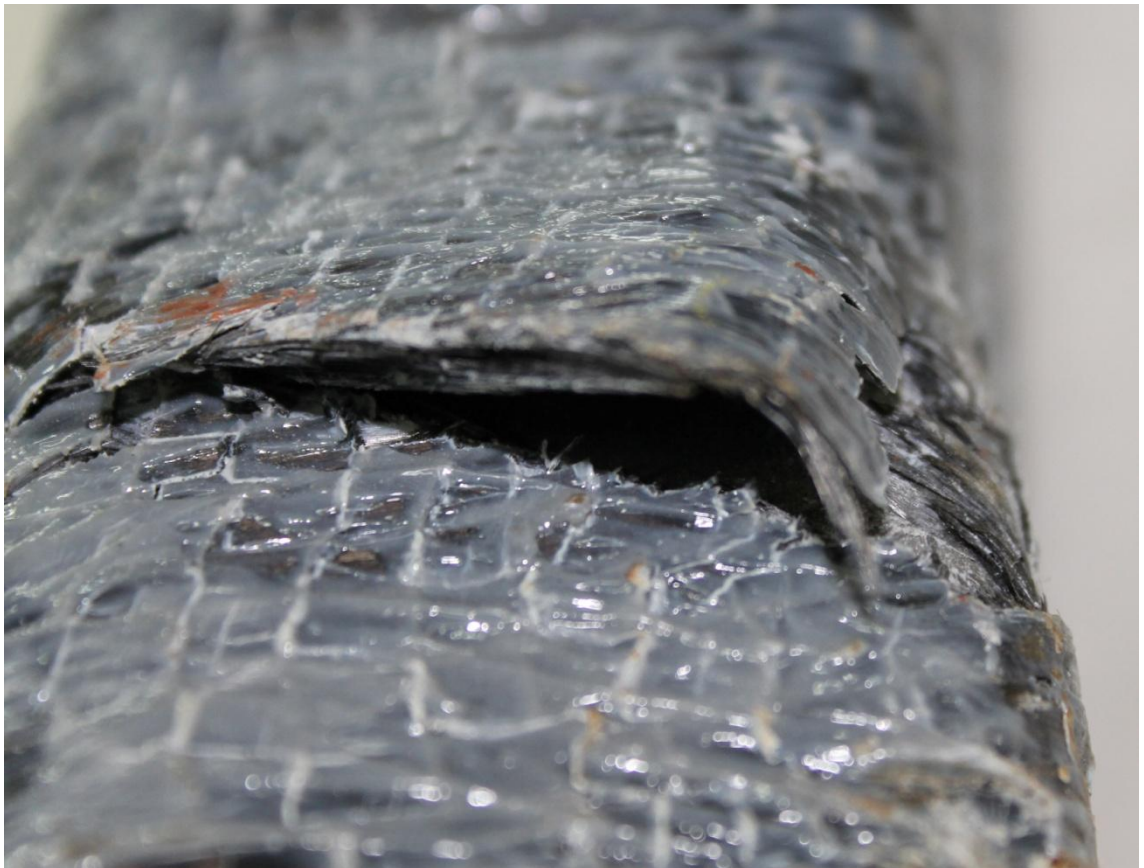
Figure B.8 CFRP rupture and debonding failure mode of SHS1 RRRS60°
