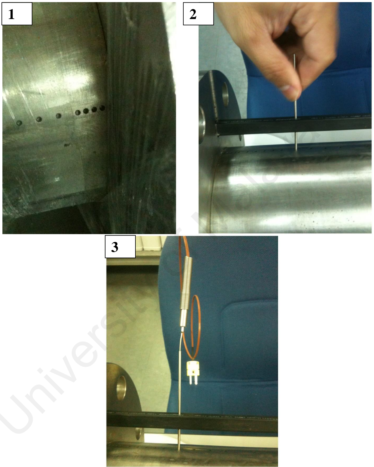
Figure 4. 3: The steps of make grooves and fixing thermowalls and installing thermocouples on the surface of the test section.
