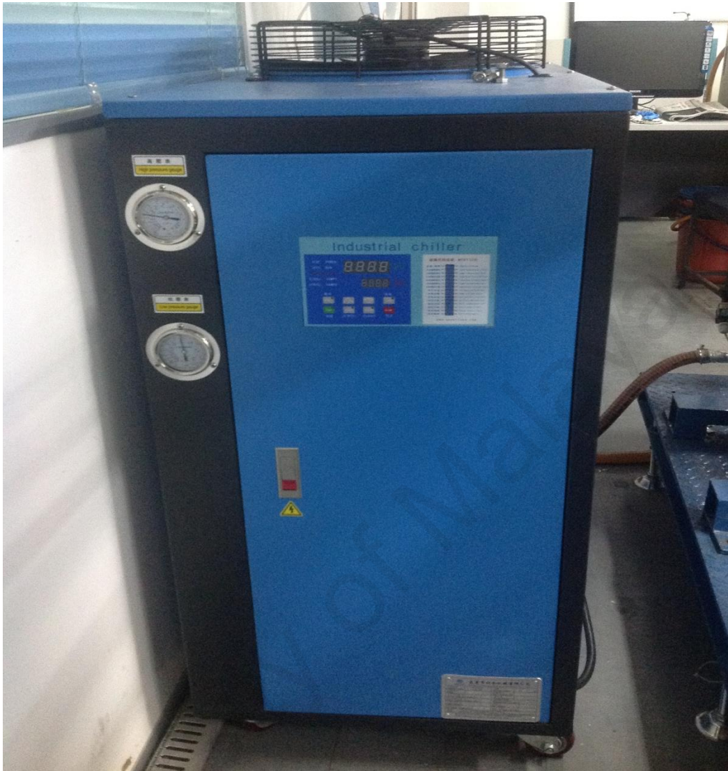
Figure 4. 5: Water cooling chiller.
