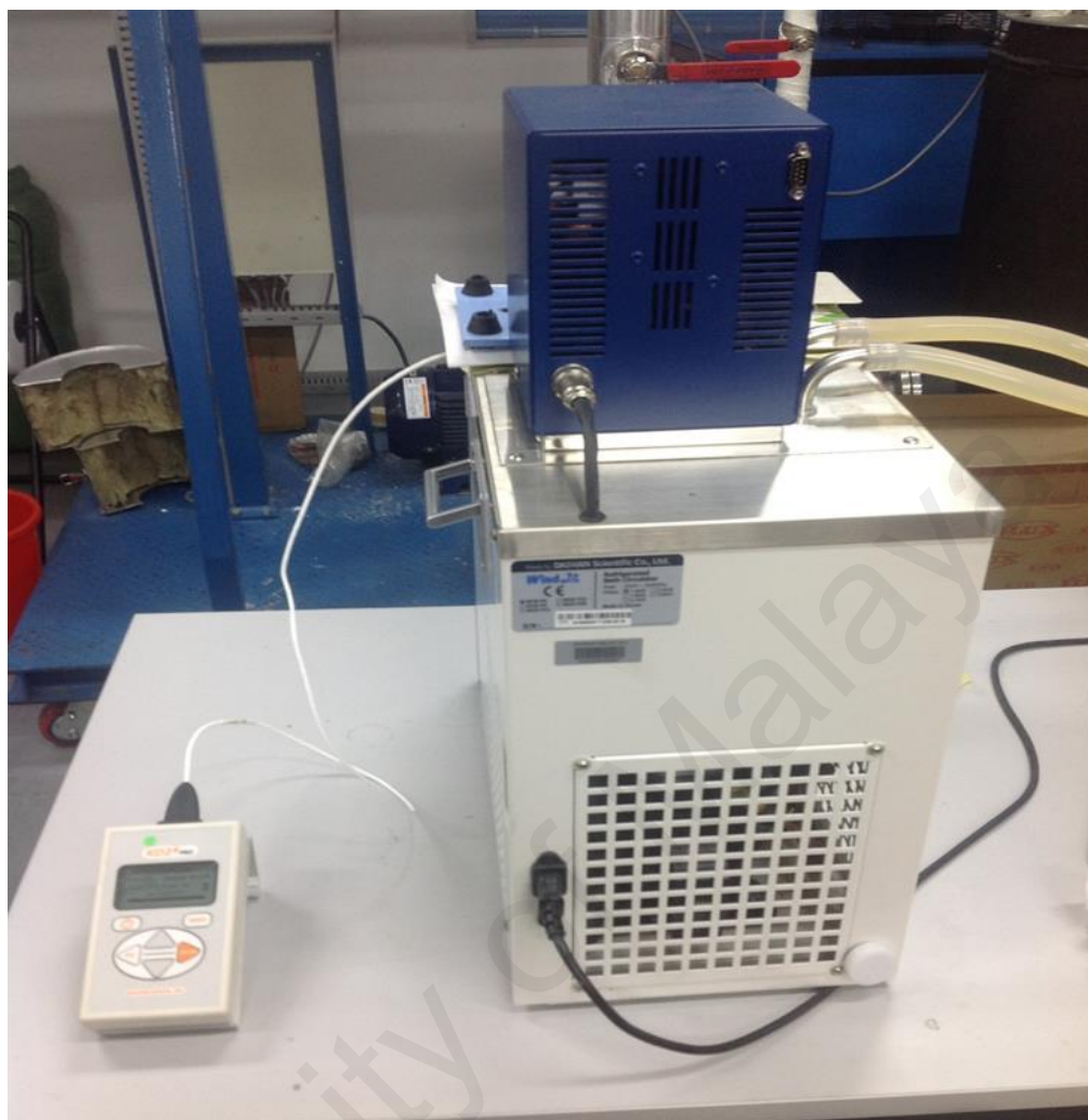
Figure 5. 4: KD2 Pro thermal analyzer and water bath
