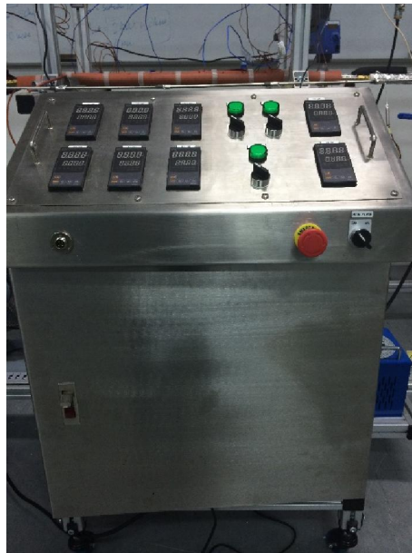
Figure 3.18 Photograph of the controlling unit that attached with sacada system
