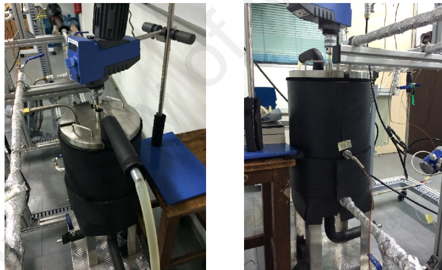
Figure 3.6 Photograph of the Reservoir Tank
