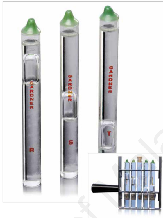
Figure 2.12 The bubble viscometers (Shames, et al., 1982)
