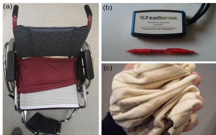
Figure 0-1: a) the placement of Texicare map on wheelchair cushion, b) The device that connected to Texicare map, c) Texicare textile. Adapted from “TexiCare: An innovative embedded device for pressure ulcer prevention. Preliminary results with a paraplegic volunteer”, by Olivier Chenu, Nicolas Vuillerme, Marek Bucki, Bruno Diot, Francis Cannard, Yohan Payan, 2013, Journal of tissue viability , 22
