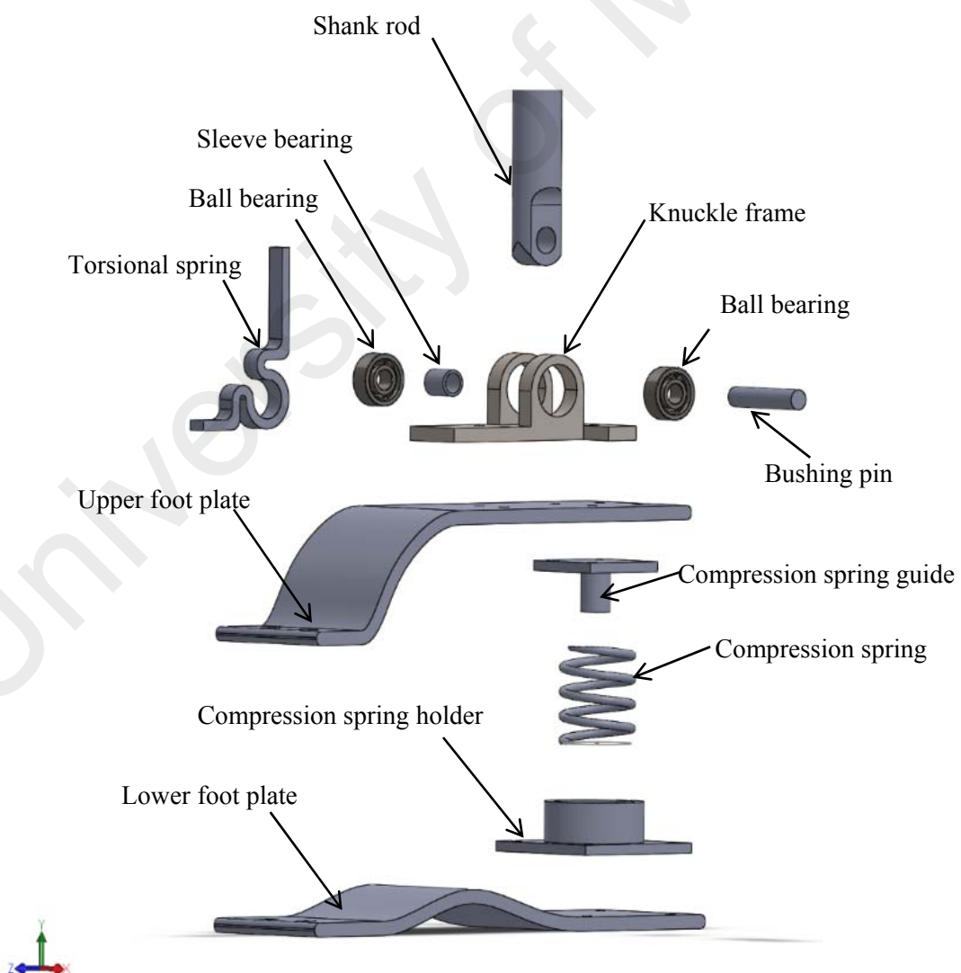
Figure 4.9: The exploded view of the different ankle joint components.
