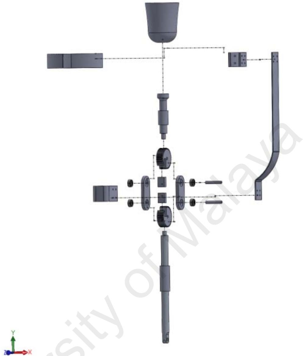
Figure 4.4: The exploded view of knee joint showing the connections among components.
