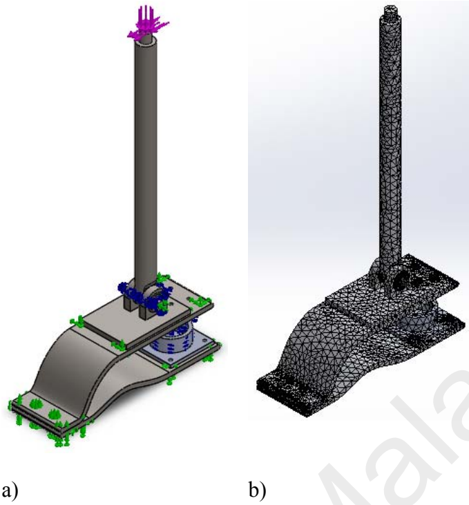
Figure 5.17: a) Model of spring based ankle joint, b) Solid mesh of the model.
