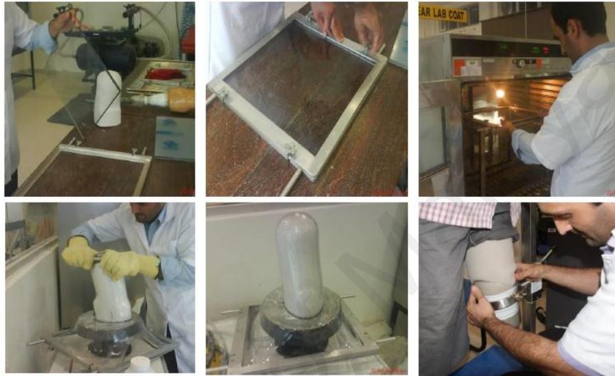
Figure 3.6: Procedures of making checking socket
