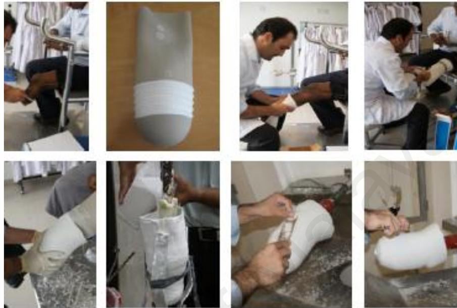
Figure 3.5: The casting and modification process
