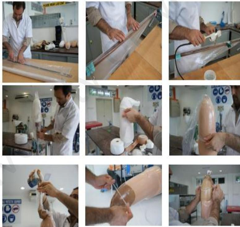
Figure 3.8: Process of making the socket with epoxy resin
