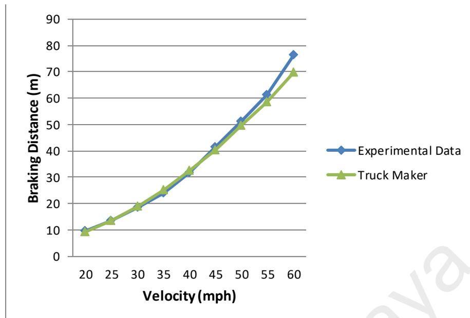
**Figure 3.2: Braking distance data comparison between experimental and simulation.**
