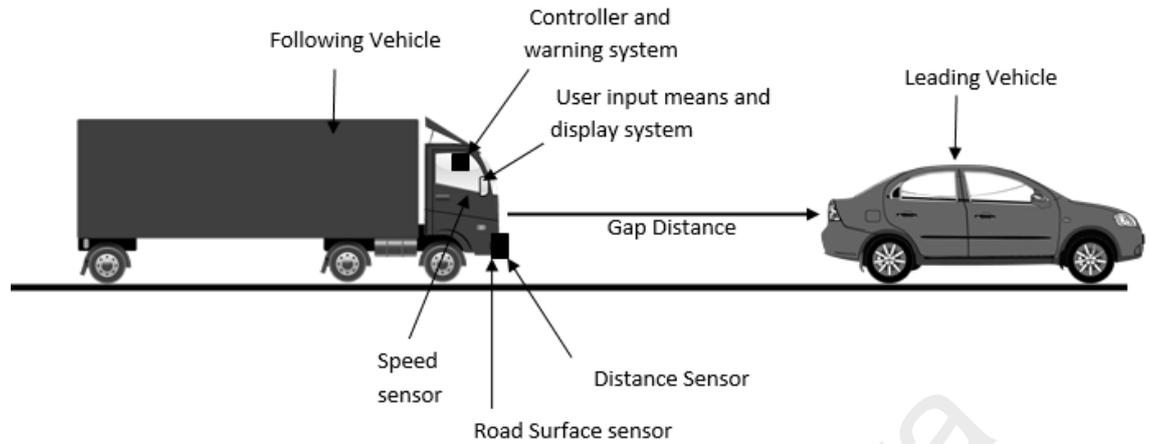
Figure 6.1: The Application of the CAWS featuring MSDG algorithm
