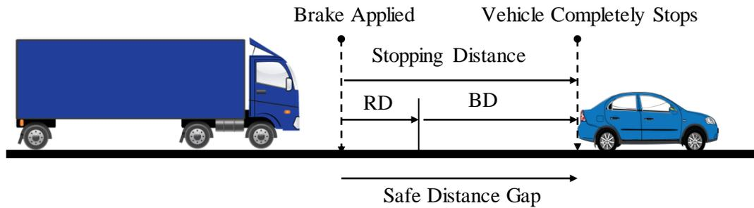
**Figure 1.4: Concept of Braking Distance and Stopping Distance**
