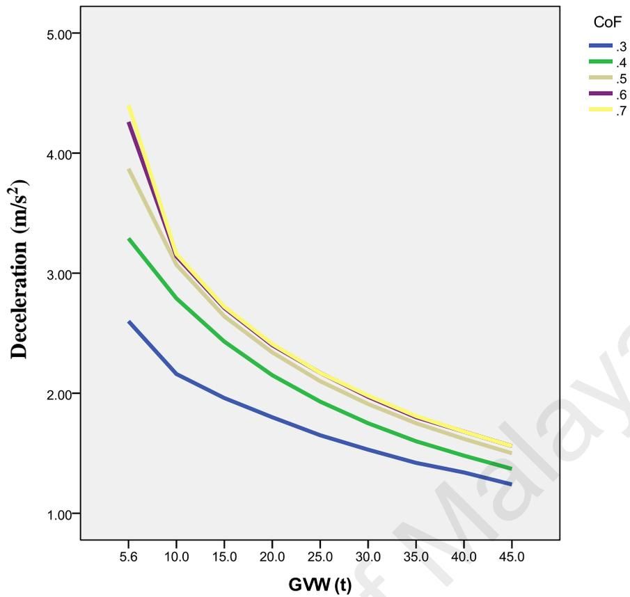
Figure 5.2: Two Axles, Deceleration vs. GVW for Speed = 11.11m/s (40km/h)
