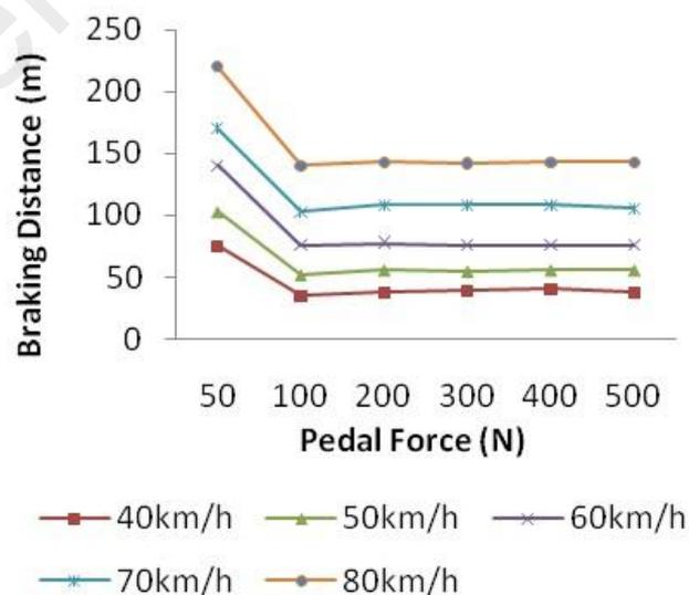
**Figure 3.5: Braking Distance for Difference in Braking Force (Sharizli 2015)**
