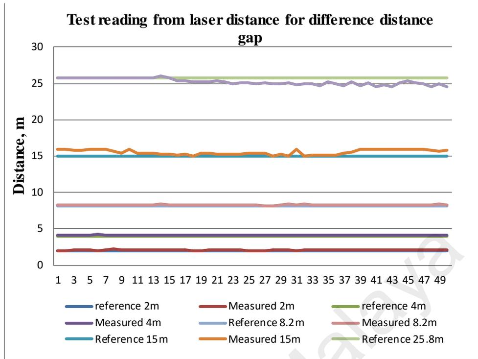
**Figure 5.22: Distance Gap Measurement Using Manual and Laser Sensor**
