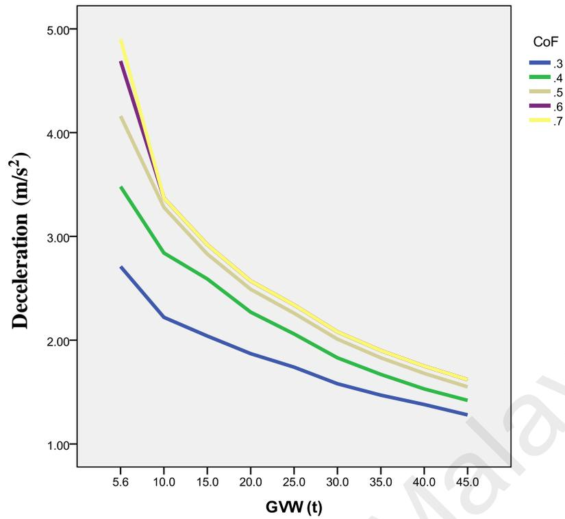
Figure 5.6: Two Axles, Deceleration vs. GVW for Speed = 22.22m/s (80km/h)
