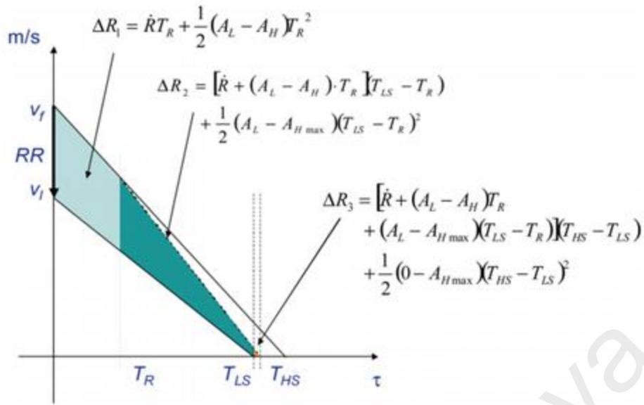
**Figure 2.5: JHU-APL Algorithm for  $T_{LS} \geq T_R$  (Brunson et al., 2002)**
