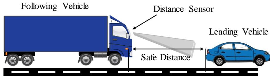
**Figure 1.3: Overall Concept of Collision Avoidance Warning System**
