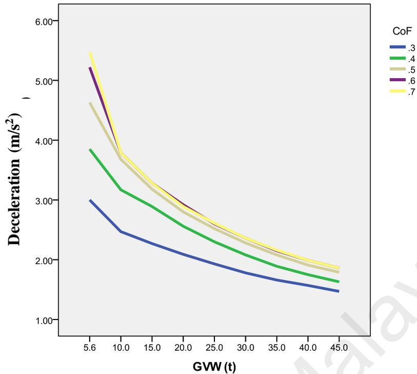
**Figure 5.8: Two Axles, Deceleration vs. GVW for Speed = 27.78m/s (100km/h)**
