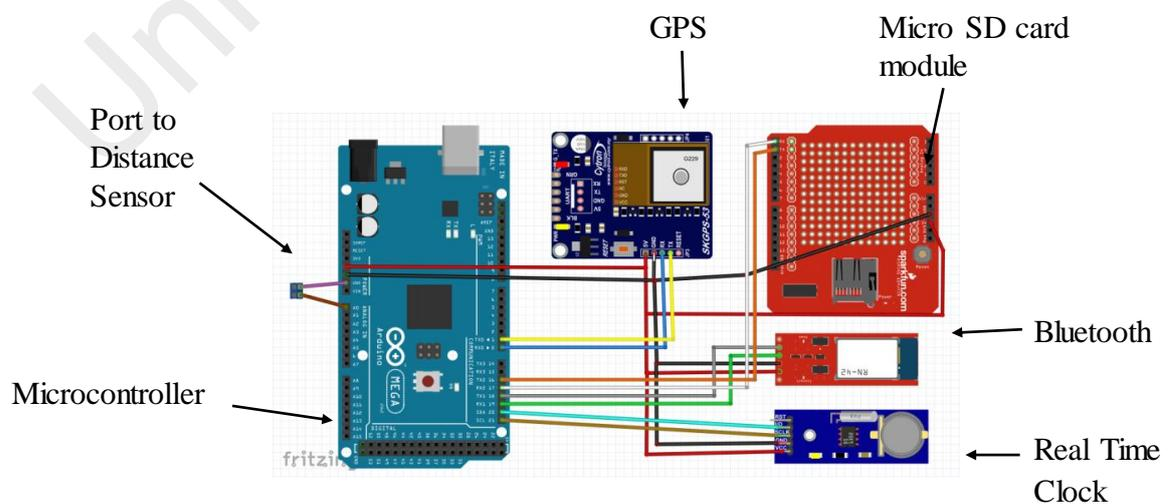
Figure 5.19: CAWS Data Logger Circuits
