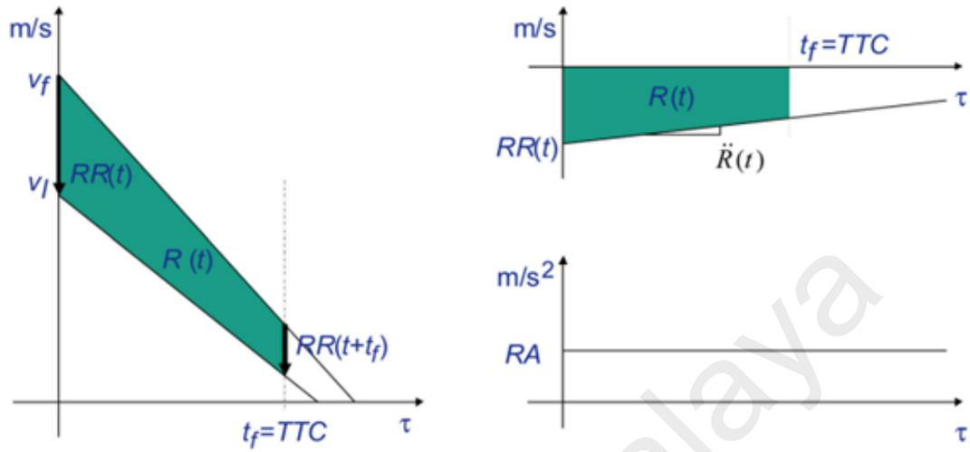
**Figure 2.4: Concept of Jaguar's Collision Warning Logic for Moving Targets (Lee and Peng, 2007).**
