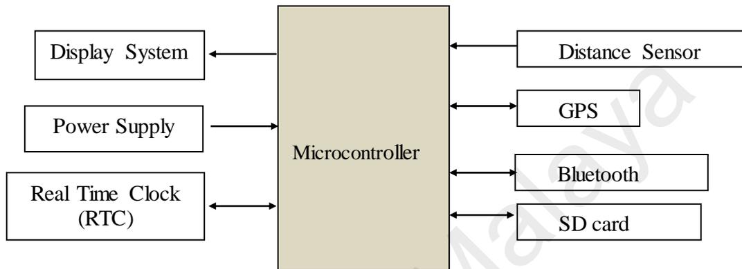
Figure 4.4: Hardware Framework of System
