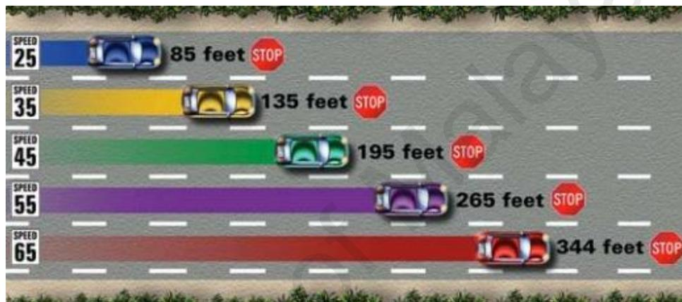
**Figure 1.5: Average Stopping Distance on Dry, Level Pavement (VTRC, 2001)**
