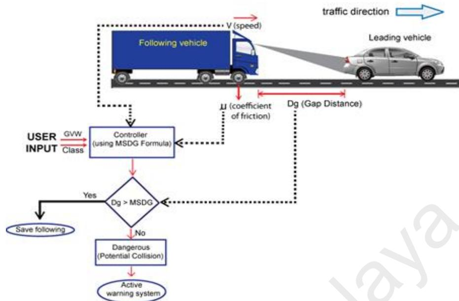
Figure 5.18: CAWS System Block Diagram
