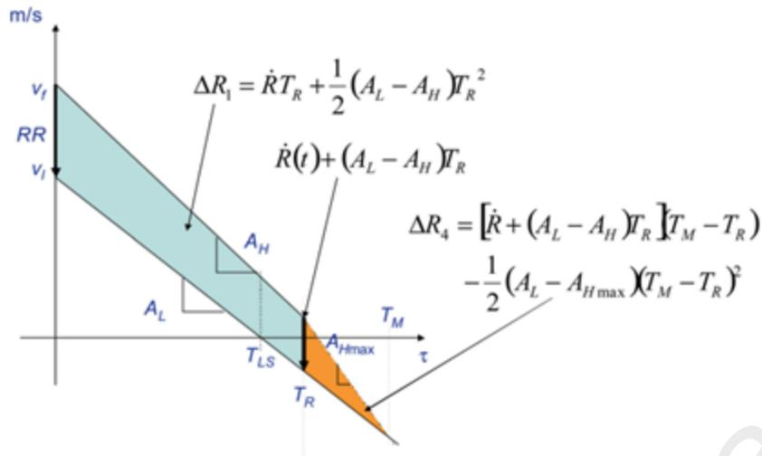
Figure 2.6: JHU-APL Algorithm for  $T_{LS} < T_R$  (Brunson et al., 2002)
