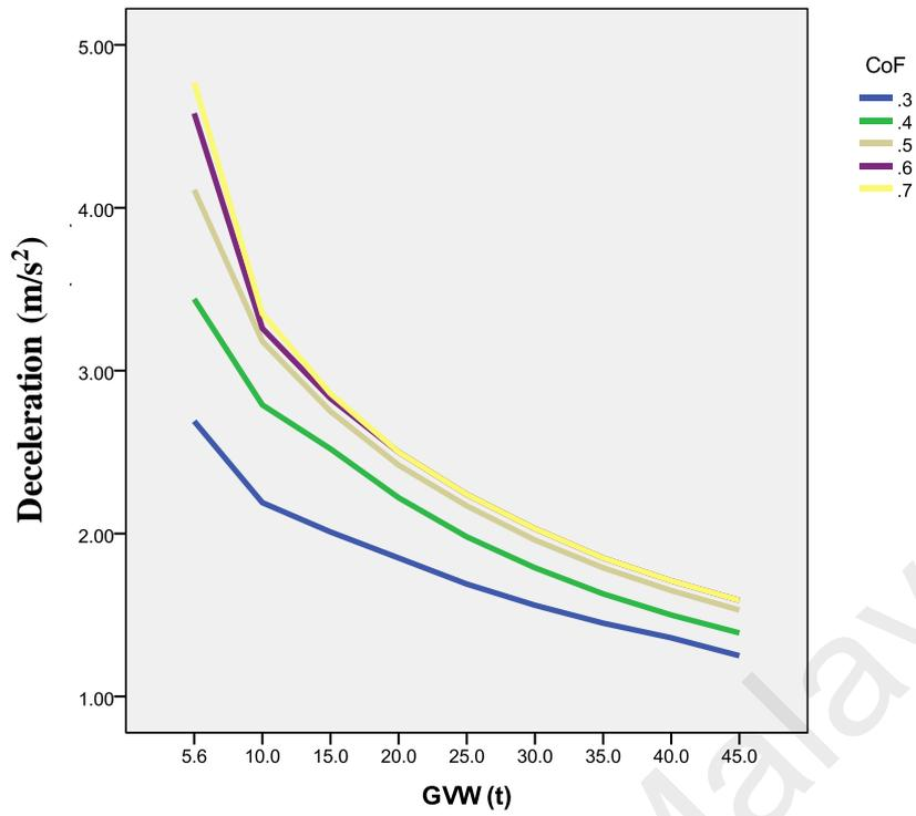
Figure 5.4: Two Axles, Deceleration vs. GVW for Speed = 16.67m/s (60km/h)
