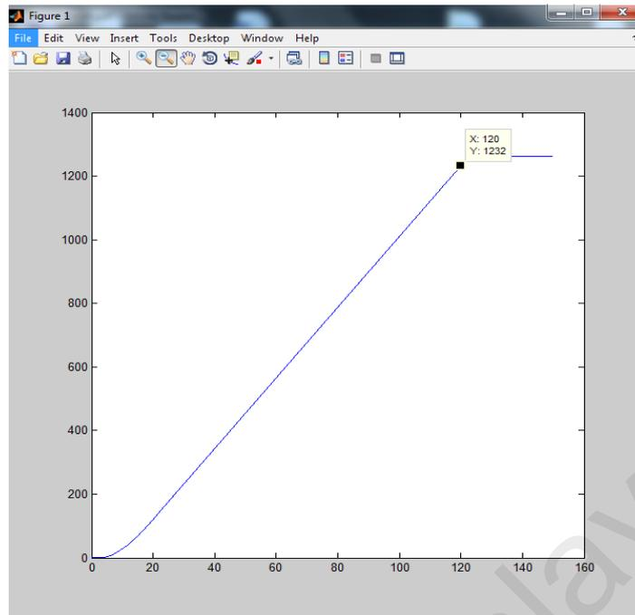
**Figure 3.8: Result in MATLAB (Start Brake Distance)**
