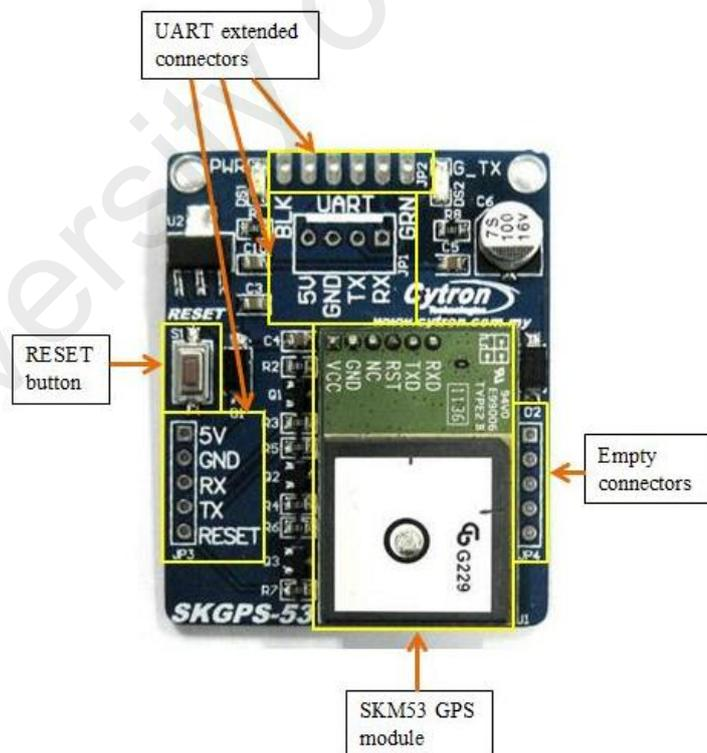
**Figure 4.9: SKGPS-53 GPS Module**
