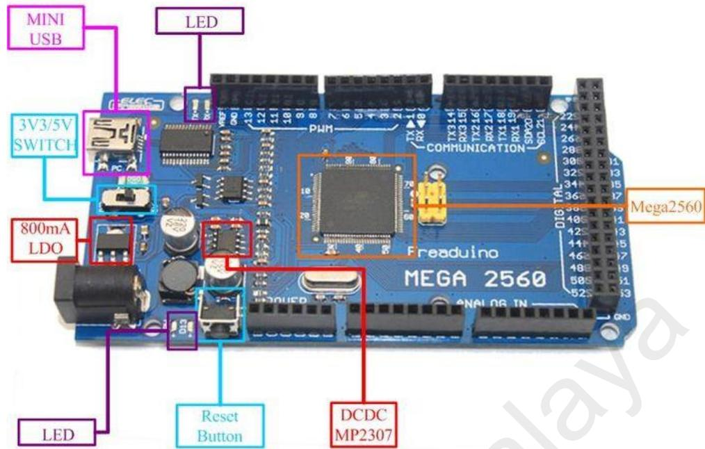
**Figure 4.5: Arduino Mega 2560**
