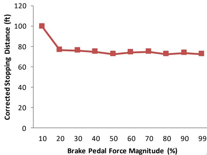
**Figure 3.6: Corrected Stopping Distance by Brake Pedal Force Magnitude for Tests Performed at 45 mph (72 km/h) (re-plotted from Gregory et al. 2010)**
