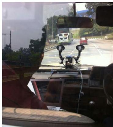
**Figure 4.17: Snap Shot System Installation In Front of Lorry**
