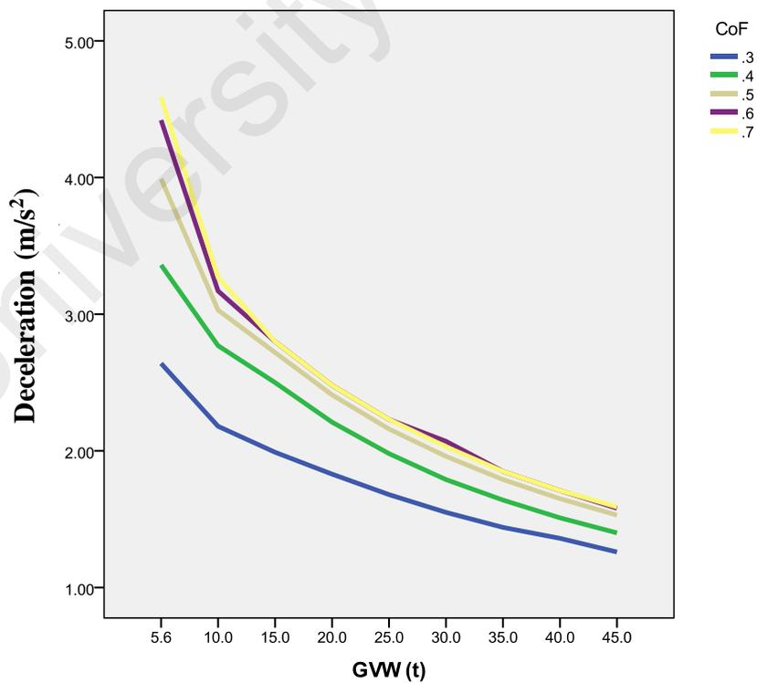
Figure 5.3: Two Axles, Deceleration vs. GVW for Speed = 13.89m/s (50km/h)
