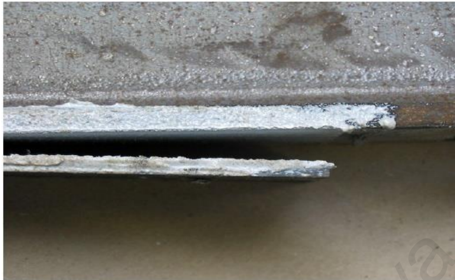
Figure 1.1: CFRP end debonding (Deng & Lee, 2007b)
