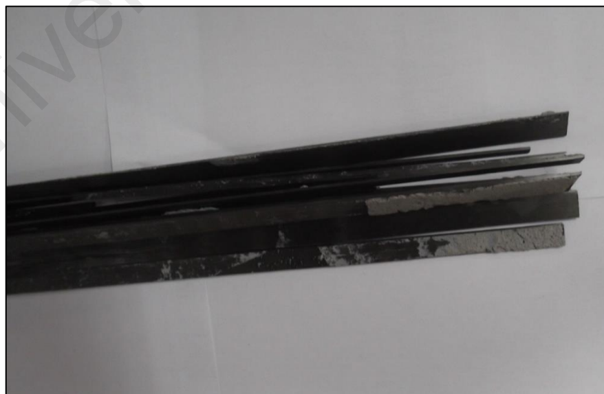
Figure 4.5: Splitting failure mode of CFRP plate (specimen M3)
