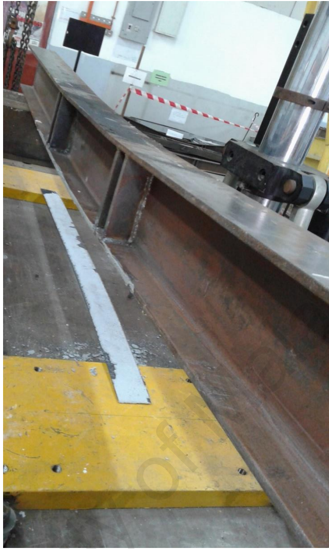
Figure 4.9: CFRP debonding failure mode of a strengthened specimen
