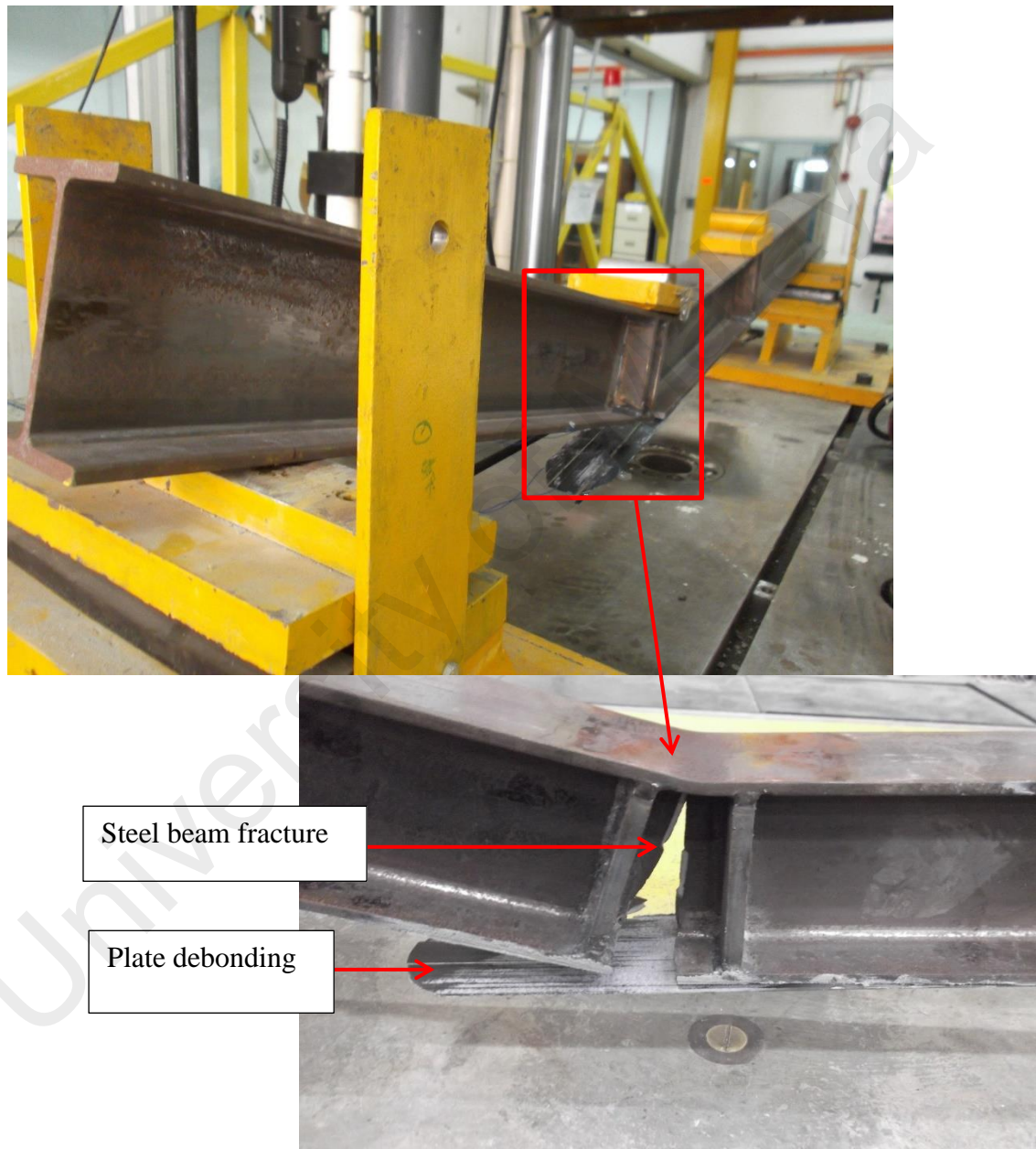
Figure 4.38: Failure mode of fatigue strengthened specimens with different in-plane CFRP end cutting shapes under fatigue
