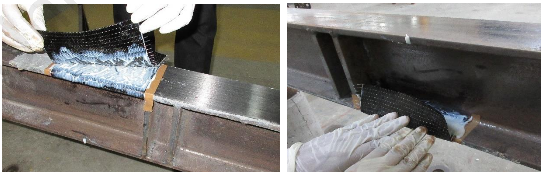
Figure 3.17: Attachment of CFRP fabrics to specimens for anchorage using adhesive
