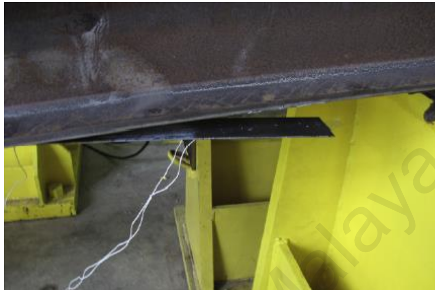
Figure 2.15: End debonding under monotonic loads
