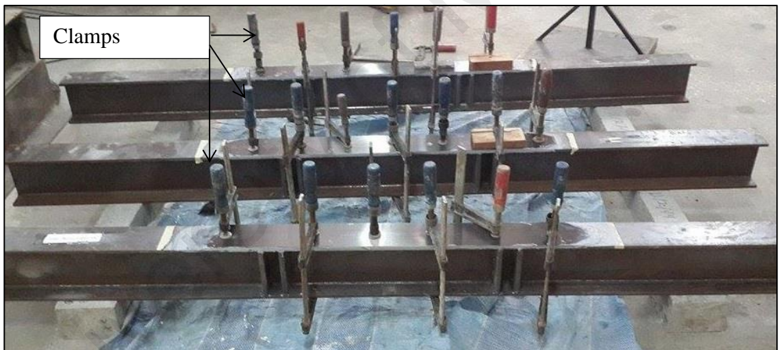
Figure 3.21: Clamping the strengthened beams using fastening clamps
