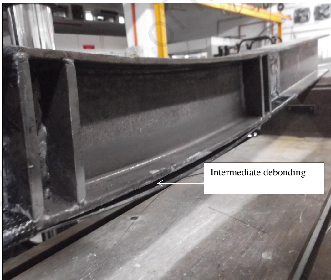
Figure 4.20: IC debonding failure mode of CFRP fabrics anchored specimens under monotonic loadings
