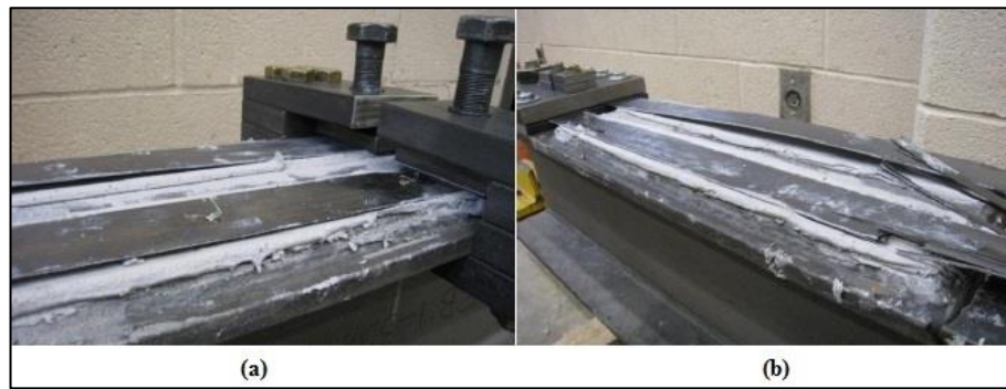
Figure 2.18: Performance of end anchorage after failure for steel beam strengthened with prestressed strips to the cover plate (a) Removable end anchor, (b) Fixed end anchor (Vatandoost, 2010)
