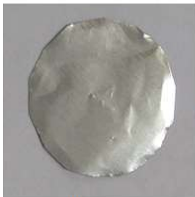
The SPE is sandwiched between the carbon electrodes (EDLC)
