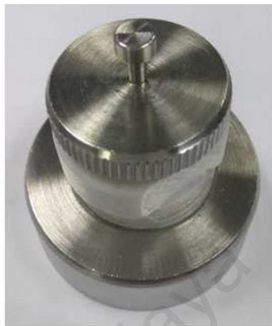
EDLC has been placed in the cell kit for electrochemical analysis
