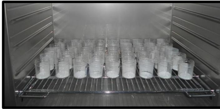
**Figure 4.13:** Drying of the substrate powders.
