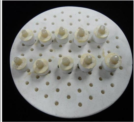
**Figure 5.7:** Samples before sintering.
