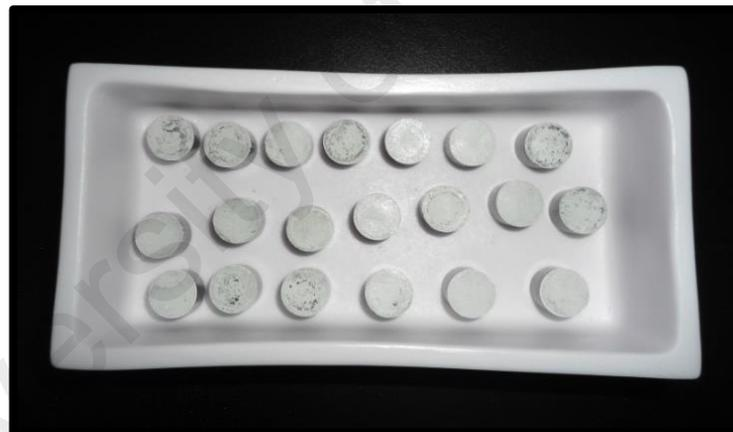
**Figure 4.22:** The graded ceramic green specimens before sintering.
