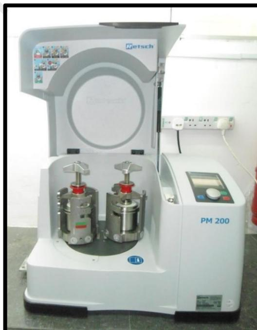
**Figure 4.15:** A planetary ball mill machine used.
