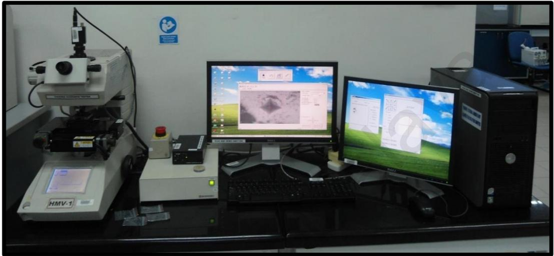
**Figure 4.28:** MicroVickers hardness testing machine used.
