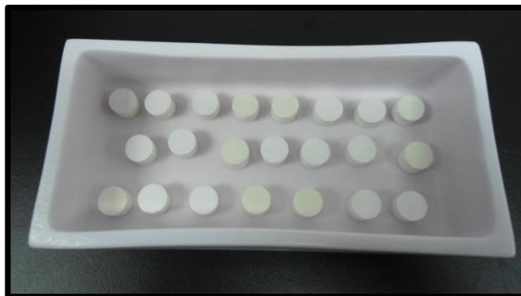
**Figure 4.23:** The graded ceramic green specimens after sintering.
