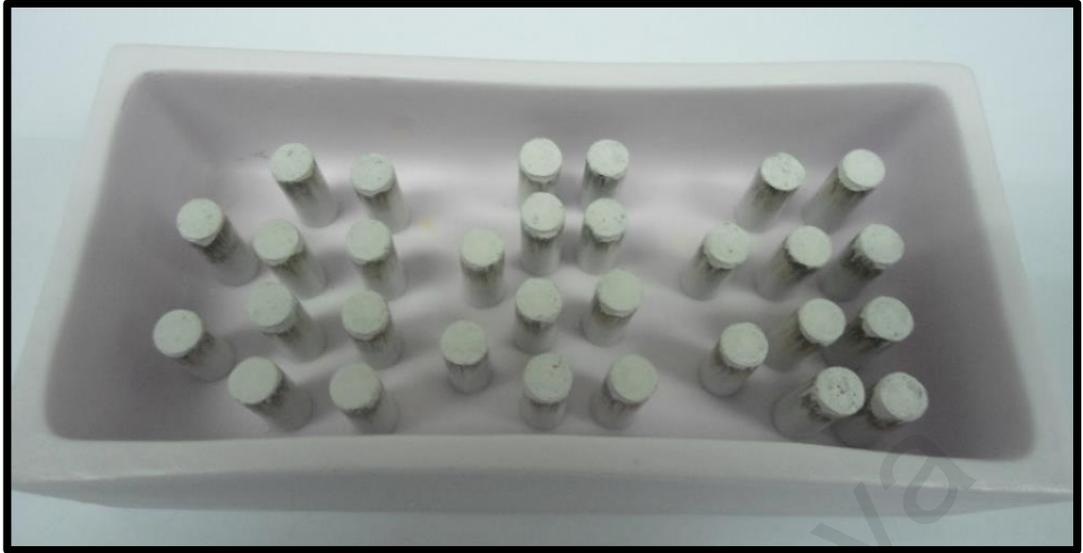
**Figure 4.30:** Specimens of ceramic cores fabricated for TMA.
