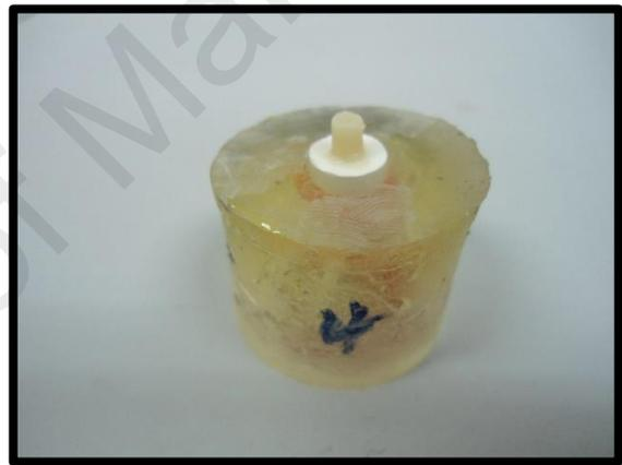
**Figure 5.13:** Specimens embedded into epoxy.
