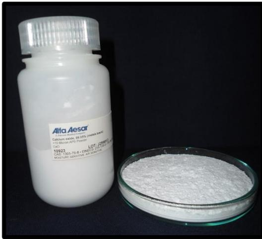
Figure 4.10: Calcium oxide (micro-size).
