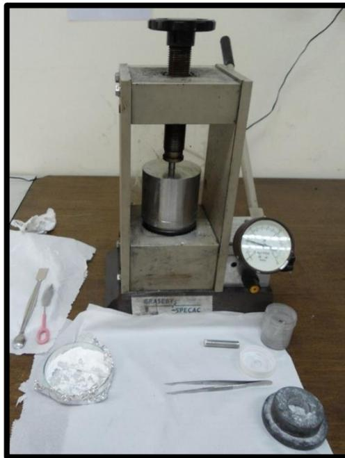
**Figure 4.18:** Uni-axial hydraulic pressing machine used.
