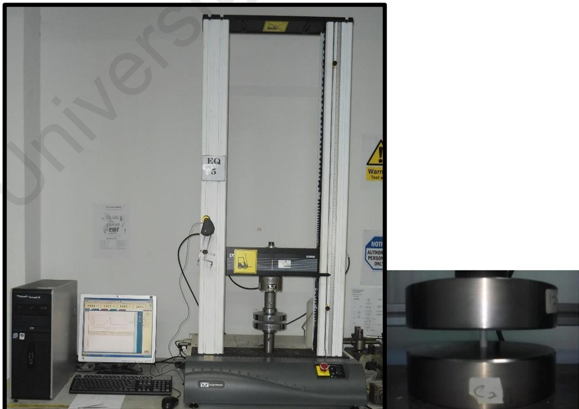
**Figure 4.29:** A universal testing machine used.
