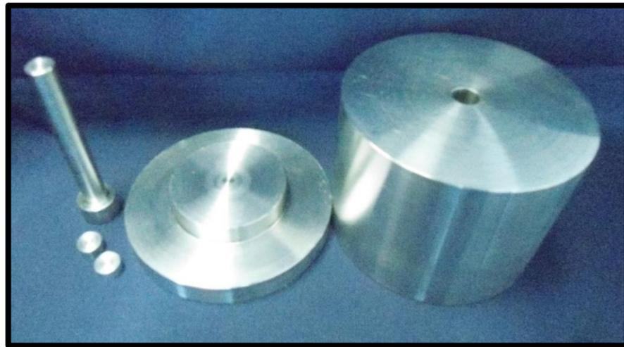
**Figure 4.16:** A custom made stainless steel compaction die used.
