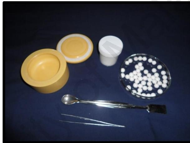
**Figure 4.14:** Zirconium jar and balls.
