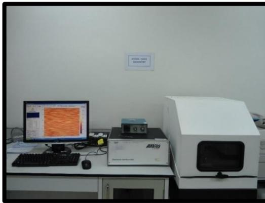
Figure 5.10: Atomic force microscope used.
