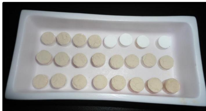
**Figure 5.2:** Infiltrated core with silica before sintering.
