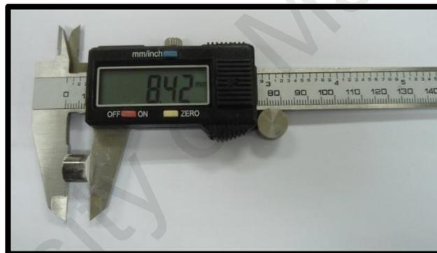
**Figure 4.19:** The graded ceramic green specimen.
