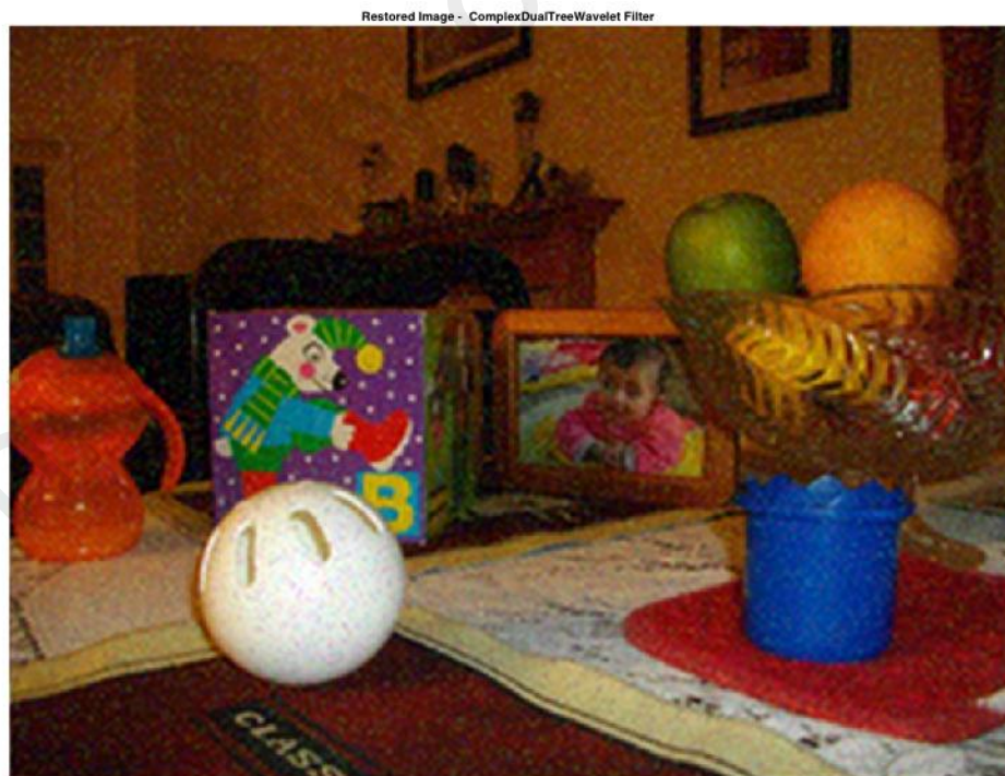
Figure 4.46 Restored Image using Complex Dual Tree Filter in the present of Salt & Pepper noise at 0.01 density.
