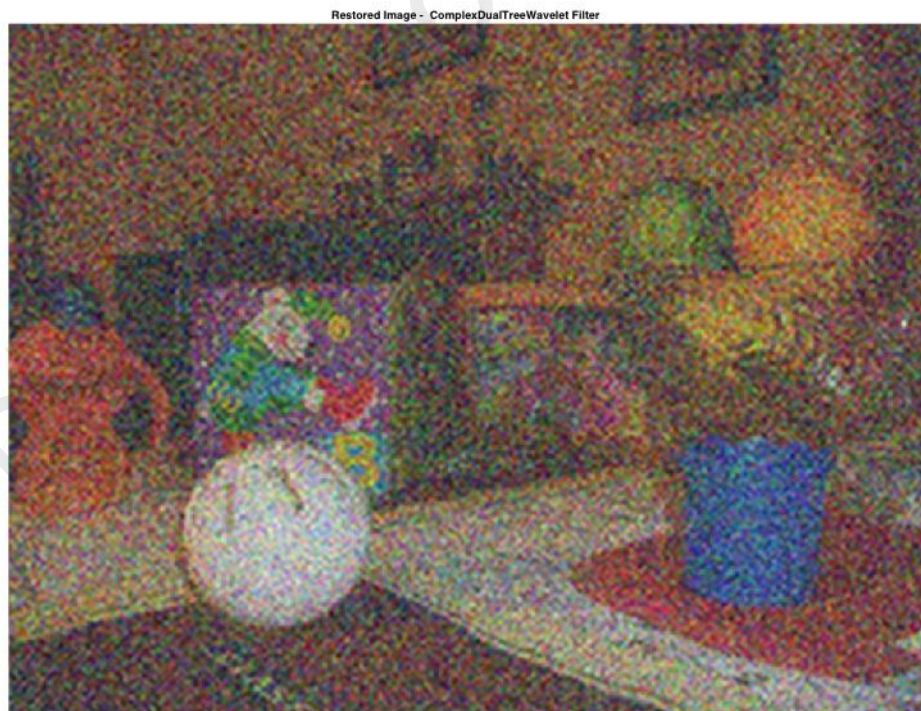
Figure 4.42 Restored Image using Complex Dual Tree Wavelet Filter in the present of Gaussian noise with 0 mean and 0.1 variance.
