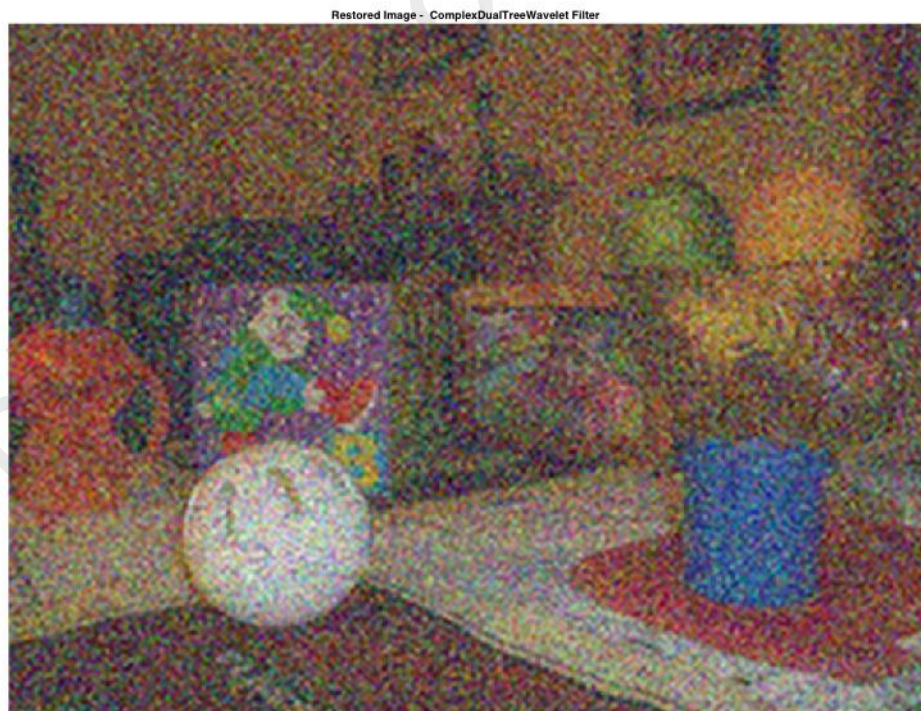
Figure 4.48 Restored Image using Complex Dual Tree Filter in the present of Salt & Pepper noise at 0.1 density.
