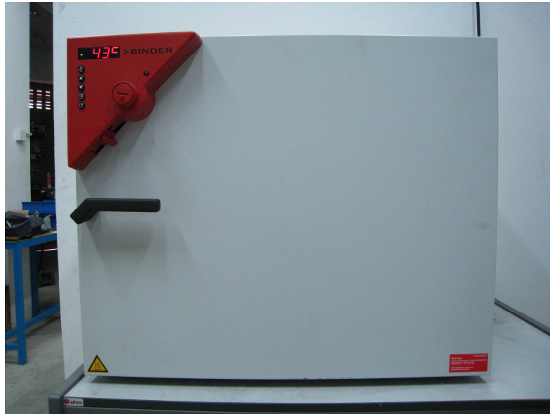
Figure 3.6: Oven for drying process of SiC particles.
