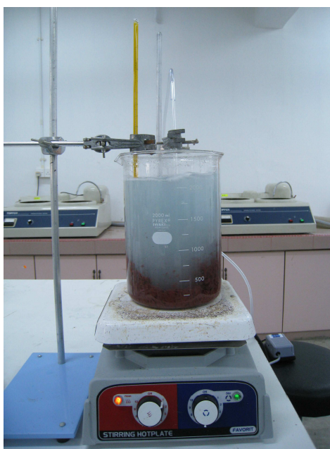
Figure 3.8: Electroless copper coating process of silicon carbide particles.
