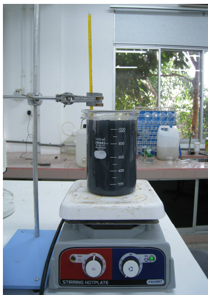
Figure 3.4: Sensitization process of SiC particles.
