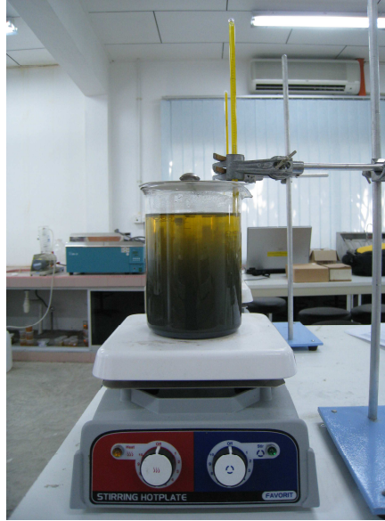
Figure 3.5: Activation process of SiC particles.
