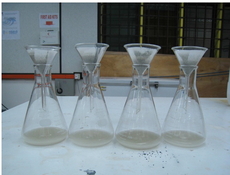
Figure 3.3: Filtering the SiC particles after ultrasonic cleaning in acetone for 15 minutes.
