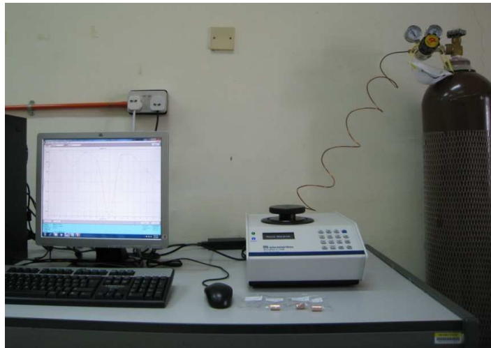
Figure 3.14: Pycnometer for true density measurement.
