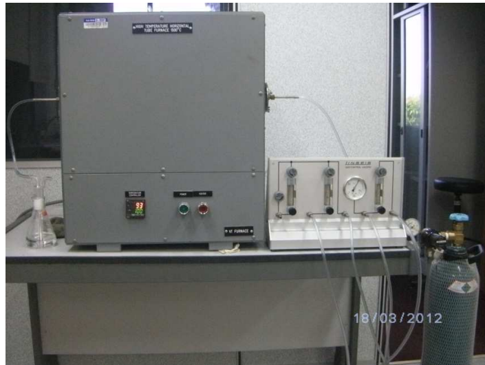
Figure 3.12: The tube furnace for sintering process.
