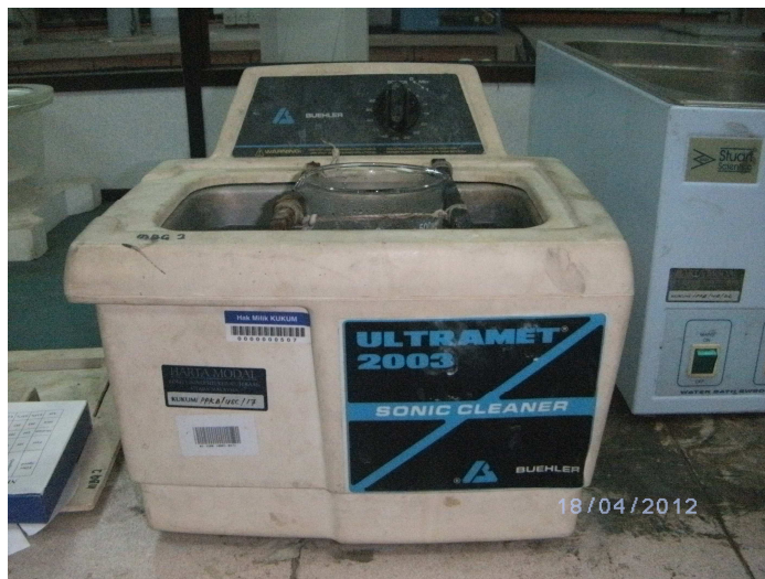
Figure 3.2: Ultrasonic cleaning of SiC particles.
