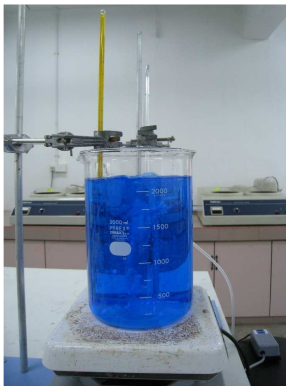
Figure 3.7: Electroless solution bath for coating process of SiC particles.
