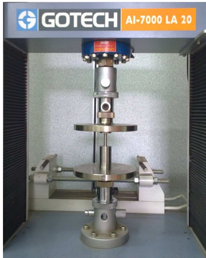
Figure 3.11: Compaction process using uniaxial Gotech 200kN UTM machine.
