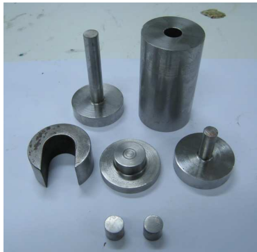
Figure 3.9: Mold and tool set used in green compaction process.
