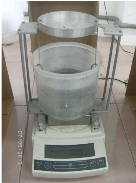
Figure 3.15: Density meter for bulk density measurement.
