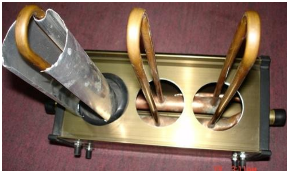
Figure 3.31 Picture of an U-pipe cross section
