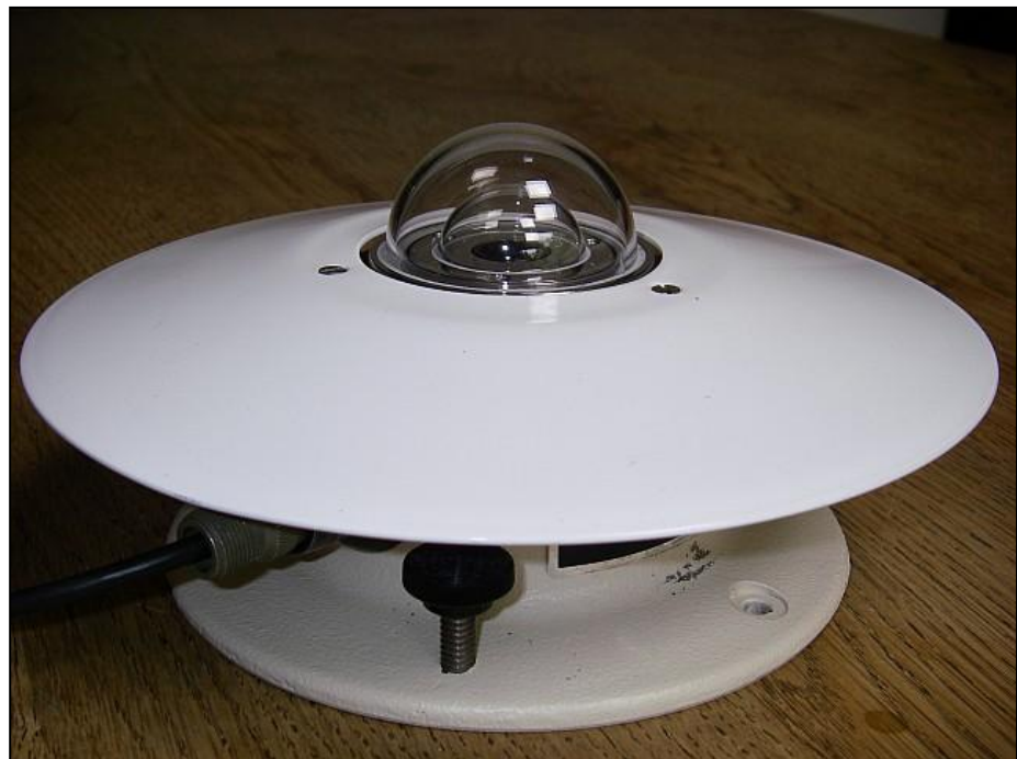
Figure 3.17 A Solarimeter, also refer to as a “Pyranometer”
