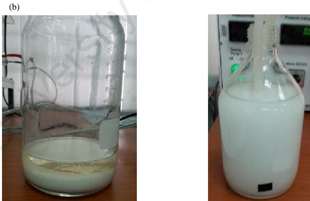
Figure 4.7: Membrane solution prepared with 0.12M Aliquat 336 and 0.18 M [Emim][NTF 2 ] : (a) 20 minutes of circulation time ; (b) 40- 80 minutes of circulation time.
