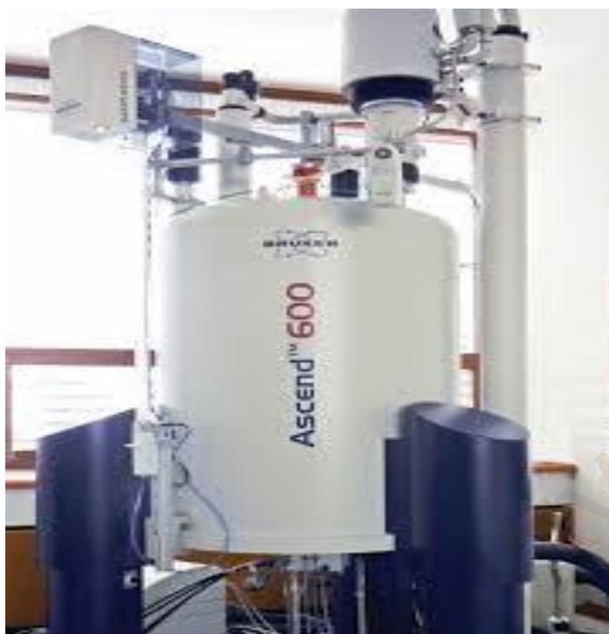
**Figure 3.9:** NMR spectrometer
