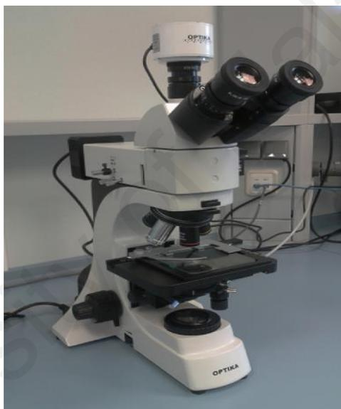
**Figure 3.4:** Optical microscope used to visualize water droplet in emulsion
