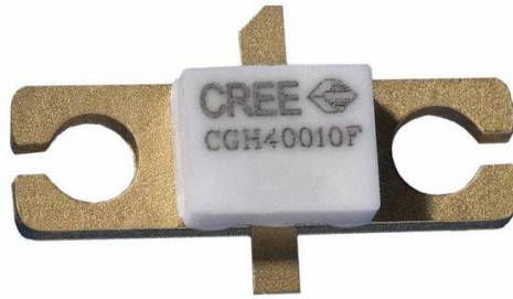
Figure 2.22: Actual component of GaN HEMT. (CREE, 2006-2007)
