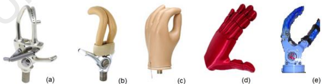
Figure 3.28: Terminal Device Tested (a) Otto Bock model 10A80 hook (Otto Bock; Duderstadt, Germany), (b) Hosmer model 99P hook (Hosmer; Campbell, California), (c) Hosmer Soft VO hand (Hosmer), (d) 3D-printed hand with 5 motors and (e) electric hand
