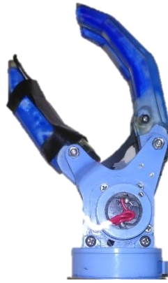
Figure 3.11: Electric Terminal Device
