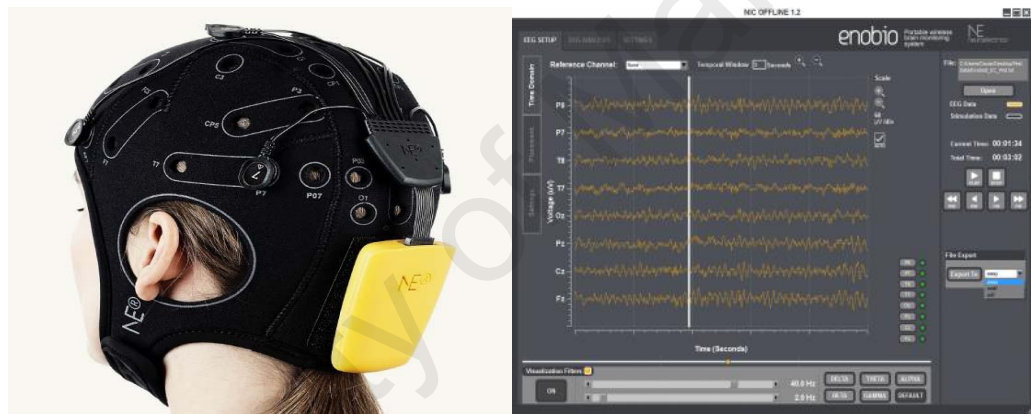
Figure 3.5: Enobio 8 Wireless EEG device and Neuroelectrics NIC 1.3 software for EEG data recording (Ruffini et al., 2007; Ruffini et al., 2006) (Adapted from http://www.neuroelectrics.com/ ).
