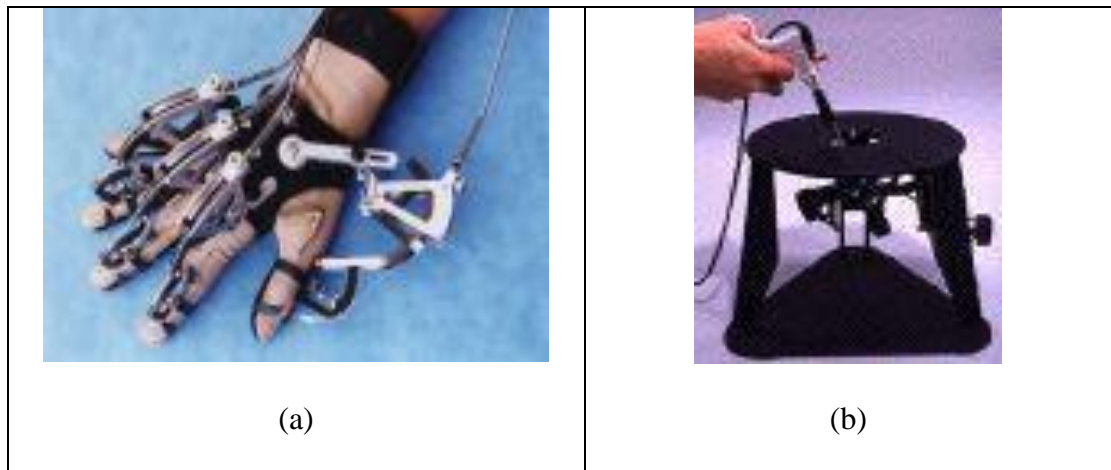
Figure 2.9: Example of haptic devices. (a) Cybergrasp Force Feedback Glove (Virtual Technologies, Inc.). (b) Laparoscopic Impulse Engine (Immersion Corporation)
