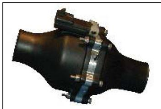
Figure 5.1 : Prototype BLDC electric water pump ( Chalgren,2004 )
