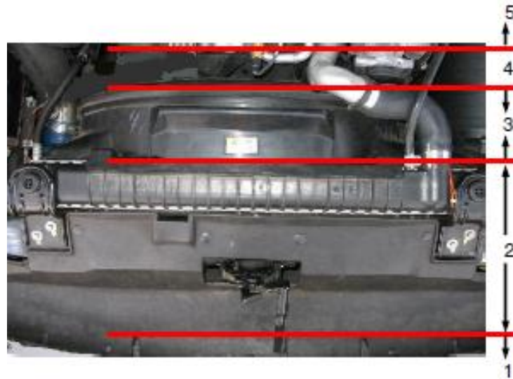
Figure 3.3 : Conventional cooling system ( 1 : inlet grill, 2 : heat exchanger pack , 3 : fan pack , 4 : room for exhaust , 5 : engine )
