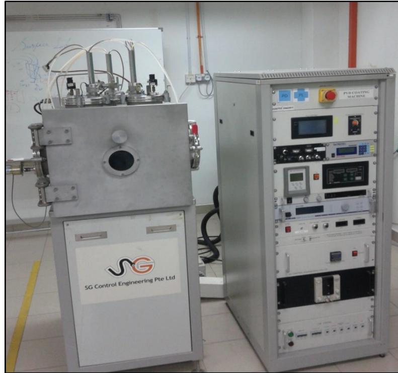
Figure 3.2: The SG Control Engineering Pte Ltd series magnetron sputtering system
