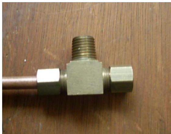
Figure 3. 5: T-socket used to join the thermocouples with the tubes.
