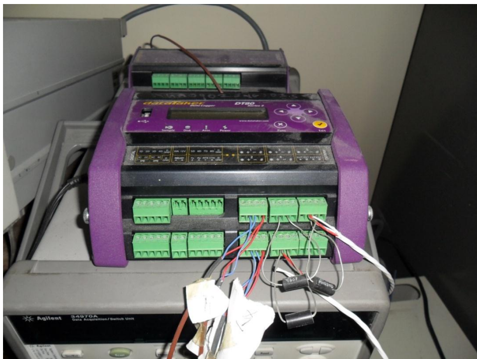
Figure 3.6: Data logger used to detect pressure and temperature.
