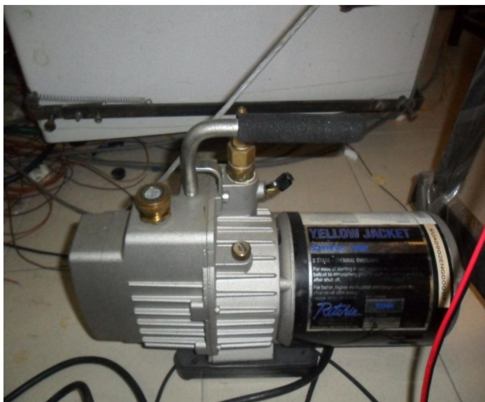
Figure 3.2: Vacuum pump for clearing the gas from the cylinder.
