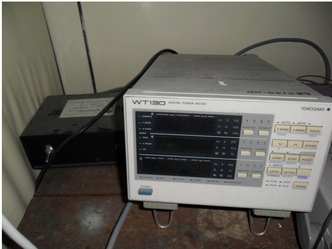
Figure 3.10: Digital power meter used to measure power consumption by the compressor.
