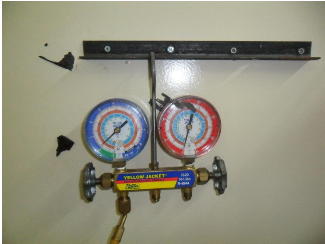
Figure 3.11:Charging hose and valve to charge and discharge the refrigerant.
