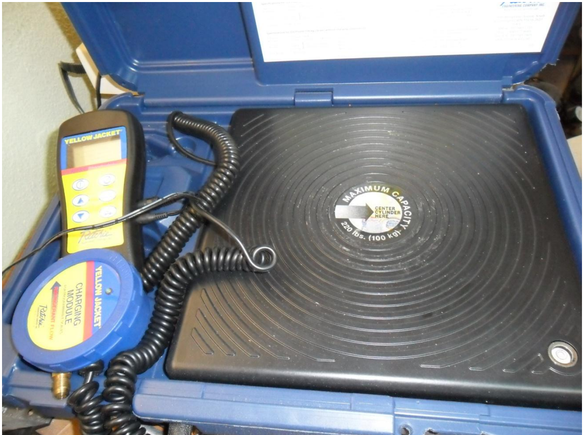
Figure 3.3: Digital electronic charging scale for charging refrigerant in the system.
