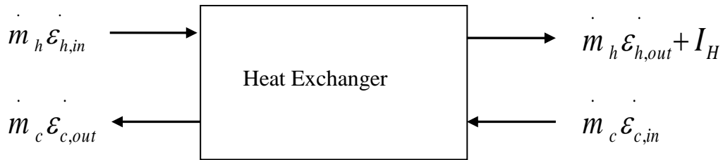
Figure 3.13 Schematic exergy flow diagram of a heat exchanger
