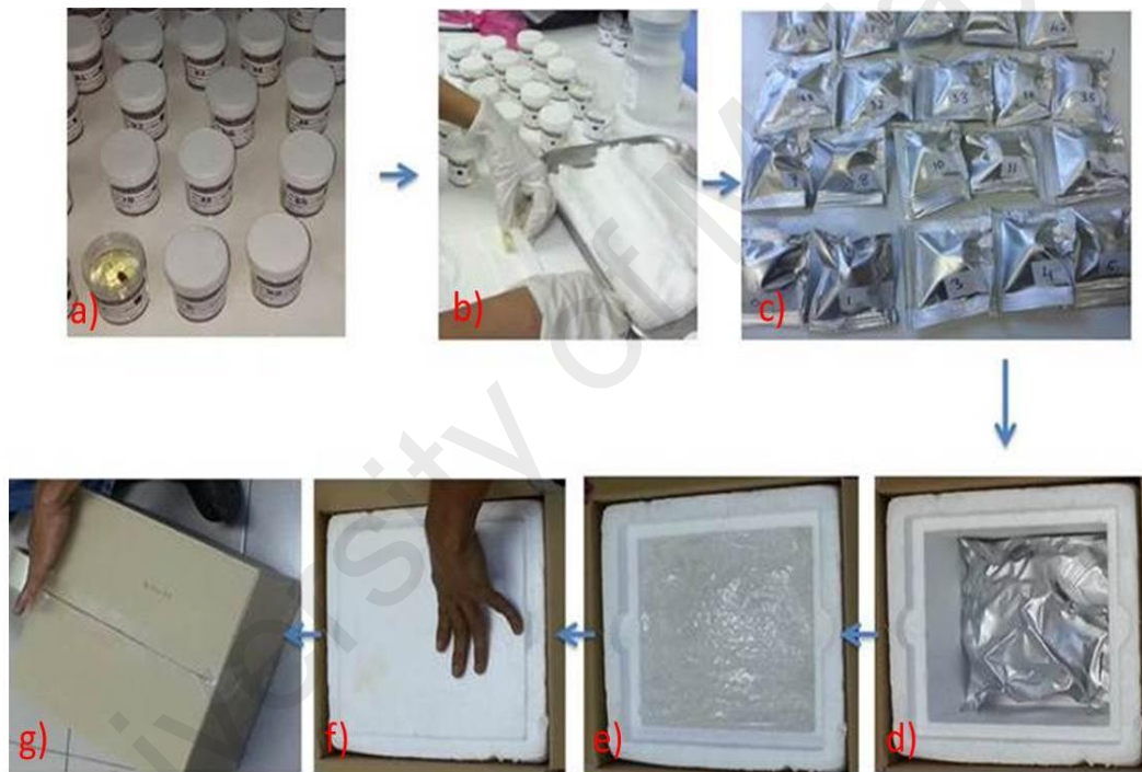
Figure 3.22: Packaging of teeth samples for Micro-CT imaging. (a) teeth samples were taken out of their respective container (b) moist cotton gauze was wrapped around each teeth sample to ensure humidity (c) each sample was packed in a small aluminum bag and sample number was written on top of each packet (d, e) all samples were prepared and then placed in one big aluminum bag which was air vacuumed and sealed (f, g) and placed in a thermocol box and sealed to avoid any damage to the samples.
