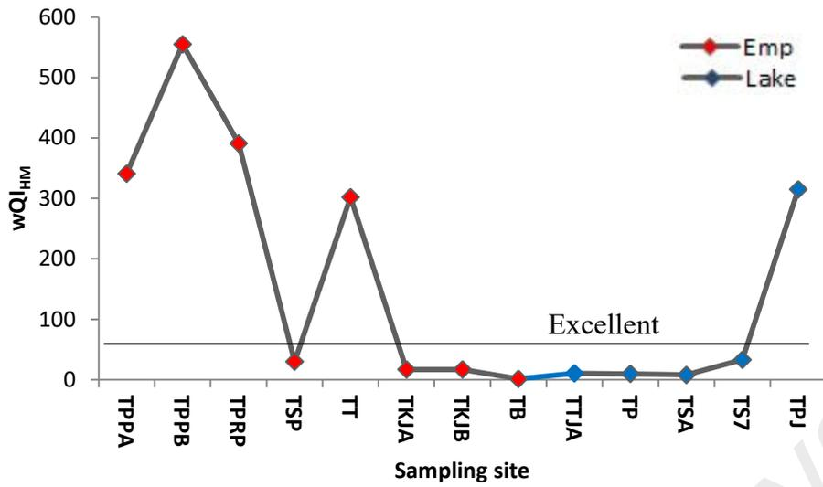
**Figure 4.23:** Heavy metals WQI<sub>HM</sub> of ex-mining ponds and lakes in Klang Valley
