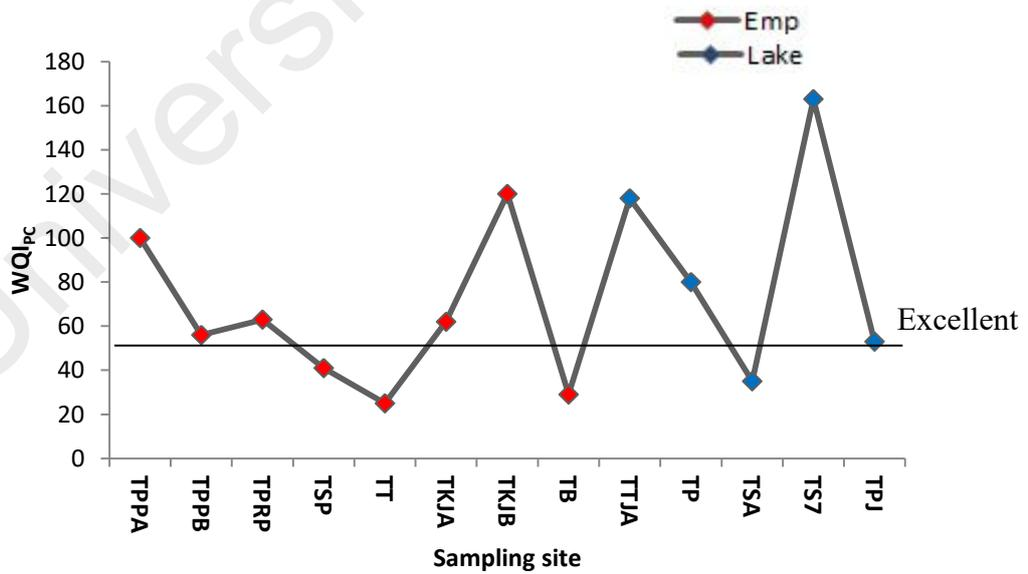
**Figure 4.24:** Physical-chemical parameter WQI<sub>PC</sub> of ex-mining ponds and lakes in Klang Valley
