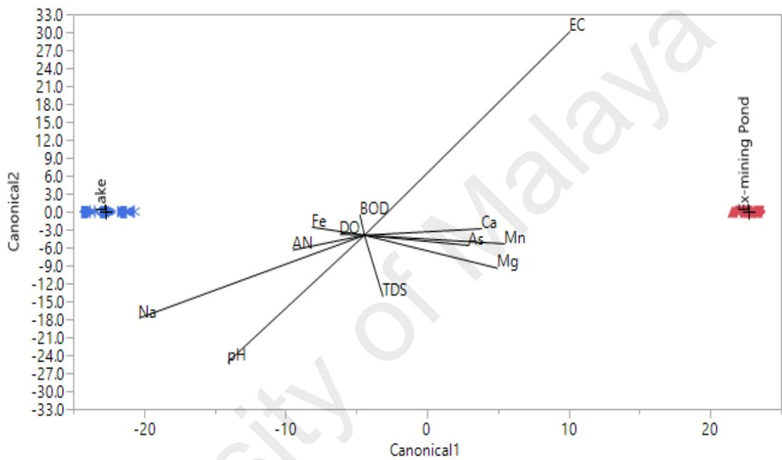
**Figure 4.8:** Canonical plot for the discrimination of water samples from ex-mining ponds and lakes in Melaka
