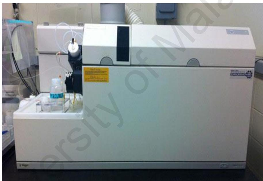
**Figure 3.1:** Inductively Coupled Plasma Mass Spectrometer (ICP-MS) (Agilent7500ce)
