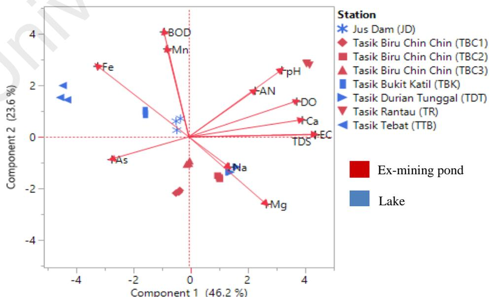
**Figure 4.6:** PCA bi-plot of metals and physical-chemical parameters in Melaka
