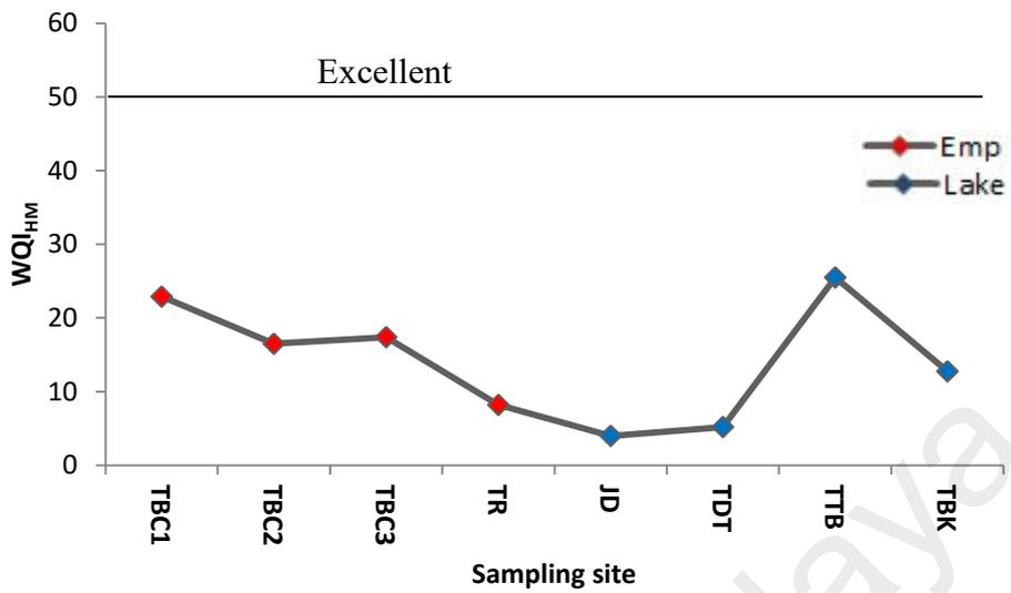
**Figure 4.25:** Heavy metals WQI<sub>HM</sub> of ex-mining ponds and lakes in Melaka
