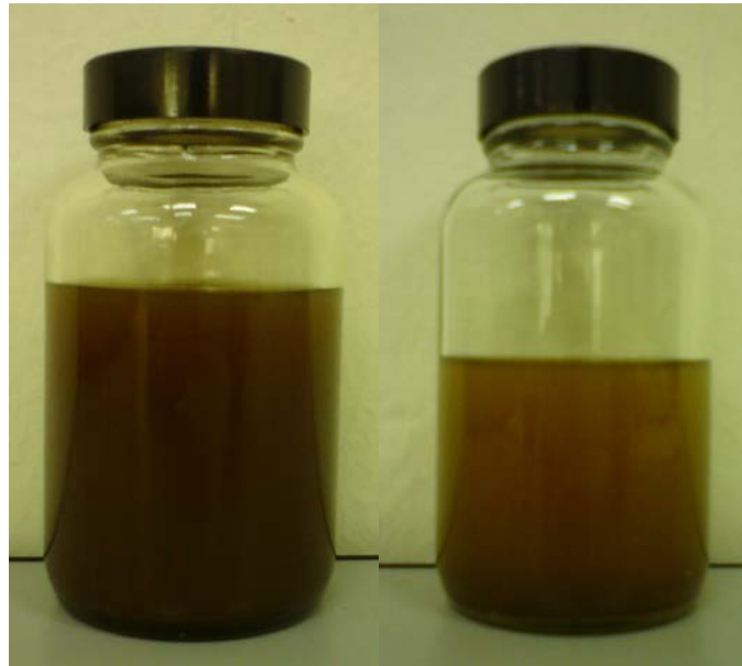
Figure 4.11: Suspension with 0.1 wt% ferrite (left) and suspension with 0.5 wt% ferrite (right).
