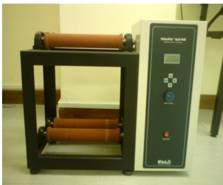
Figure 3.3: Horizontal ball mill used for homogeneous mixing in suspension.
