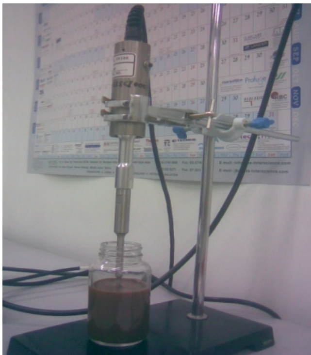
Figure 3.2: Ultrasonic probe used in homogenizing suspension.
