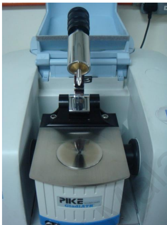
Figure 3.13 The FT-IR machine.
