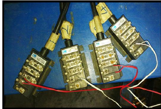
Figure 3.14: Lead wires of strain gage are connected to Wheatstone bridge.
