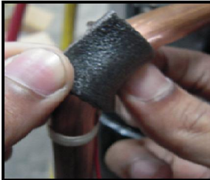
Figure 3.13: Strain gage is covered by polyethylene insulation
