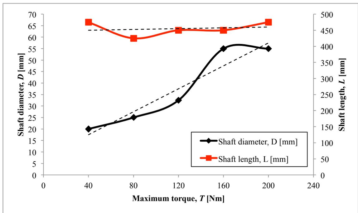
Figure 4.1 : Shaft and diameter length.
