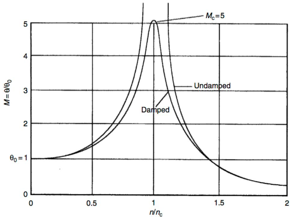
Figure 2.9 : Effect of damped and undamped vibration. [Jayabalan, 2004]
