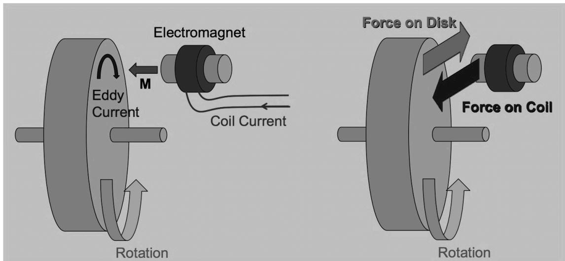
Figure 2.3 : Eddy current dynamometer. [Gitano, 2008a]
