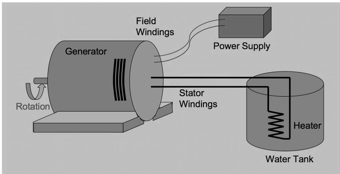
Figure 2.4 : Generator type dynamometer. [Gitano, 2008a]
