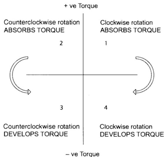
Figure 2.7 : Operating quadrants of a dynamometer. [Atkins, 2009]
