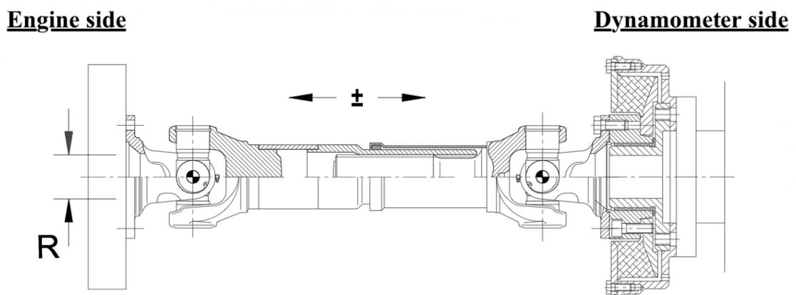
Figure 2.11 : Couplings installed on a shaft. [Ringfeder-Corp., 2006]
