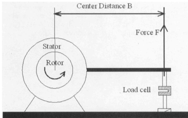
Figure 2.6 : The mechanism of torque measurement [Atkins, 2009].
