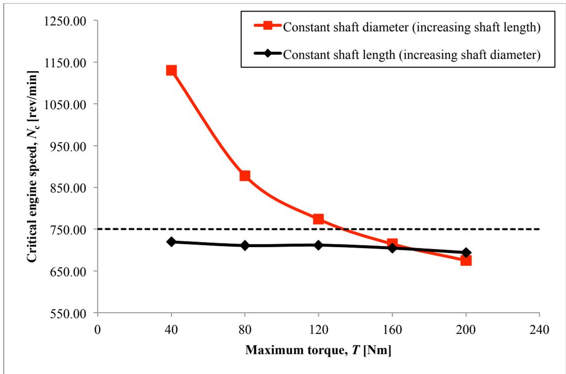
Figure 4.3 : Critical and whirling speed of the shafts with constant diameter.
