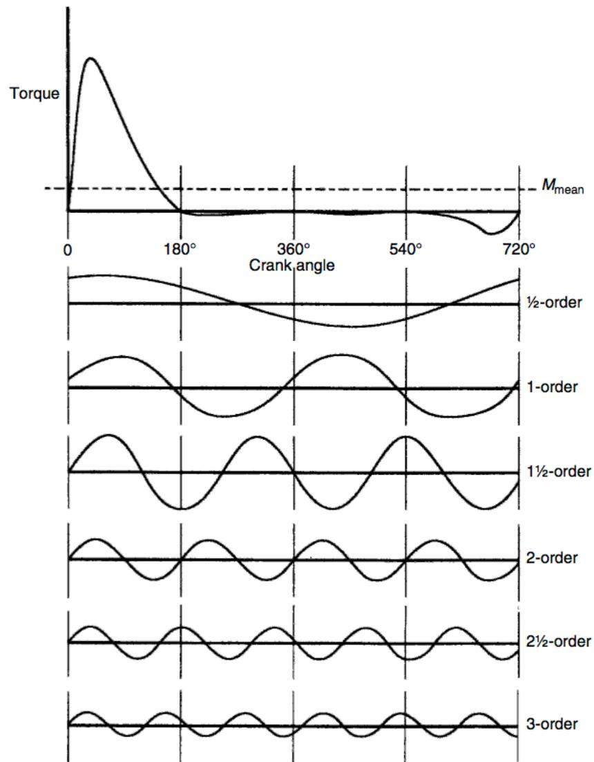
Figure 2.10 : Harmonics of engine exciting torque. [Jayabalan, 2004]
