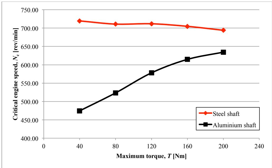
Figure 4.4 : Critical engine speed of steel and aluminium shaft.
