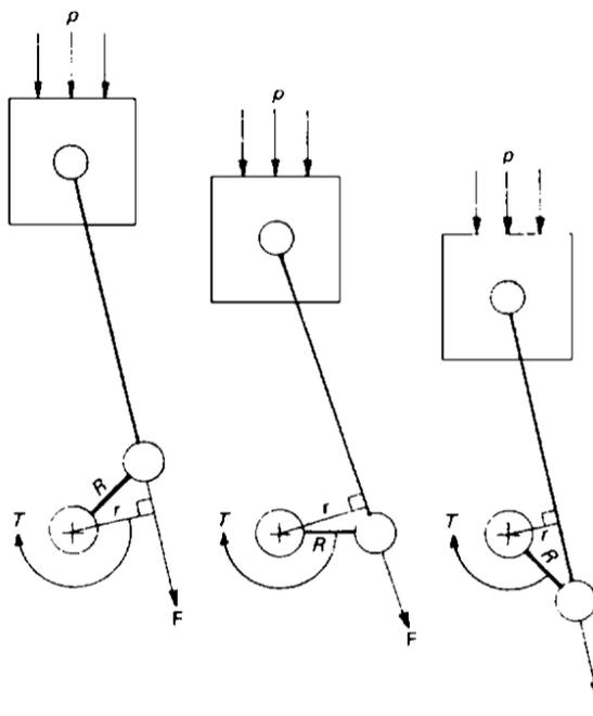
Figure 1.1 : Torque variation during power stroke. [Heisler, 1998]
