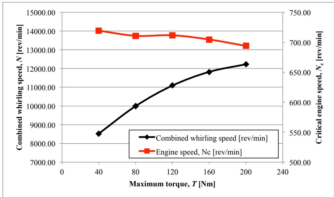
Figure 4.2 : Critical and whirling speed of the shafts with constant length.
