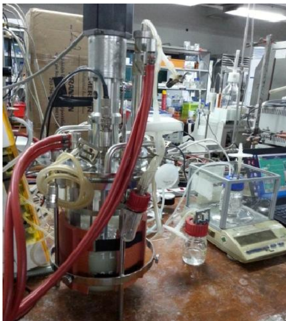
Figure 3.1: Setup of a 2-L stirred tank bioreactor for fed-batch fermentation
