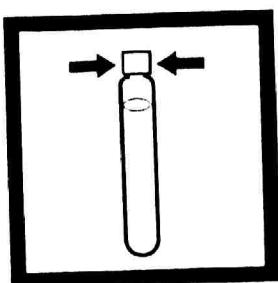
5. Replace the vial cap tightly. Use the cap tool provided, if necessary. Rinse the COD vial with demineralized water and wipe the vial clean with a paper towel.
