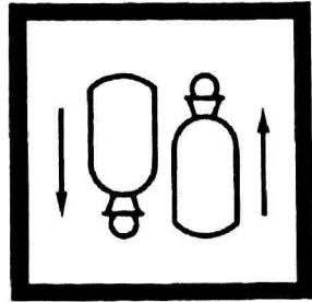
3. Immediately insert the stopper so that no air is trapped in the bottle. Invert several times to mix.
