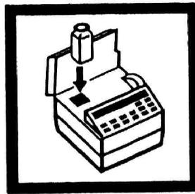
10. Within thirty minutes after the timer beeps, place the prepared sample into the cell holder. Close the light shield.
