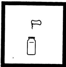
5. Add the contents of one NitraVer 5 Nitrate Reagent Powder Pillow to the cell (the prepared sample). Stopper.
