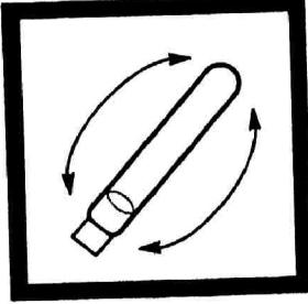
10. Invert each vial several times while still warm. Place the vials into a rack. Wait until the vials have cooled to room temperature.
