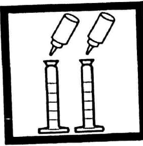
6. Add three drops of Mineral Stabilizer to each cylinder. Invert several times to mix. Add three drops of Polyvinyl Alcohol Dispersing Agent to each cylinder (hold the dropping bottle exactly vertical). Invert several times to mix.
