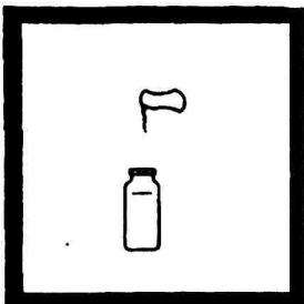
**5.** Add the contents of one PhosVer 3 phosphate Powder Pillow to the sample cell (the prepared sample). Swirl immediately to mix.
