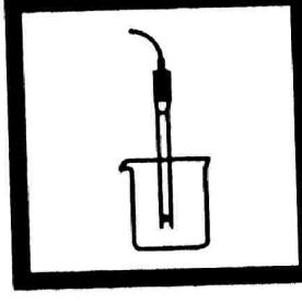
7. Place the electrode in the pH 7.00 buffer and press the Dispenser Button.
