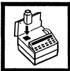
**7.** Fill another sample cell (the blank) with 25 mL of sample. Place it into the cell holder.
