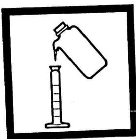
5. Fill another 25-mL mixing graduated cylinder with deionized water (the blank).
