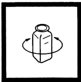
**10. Swirl the prepared sample cell to remove any gas bubbles and uniformly suspend any residue.**
