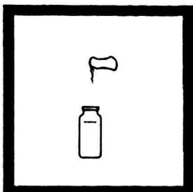
5. Add the contents of one CuVer 1 Copper Reagent Powder Pillow to the sample cell (the prepared sample). Swirl to mix.
