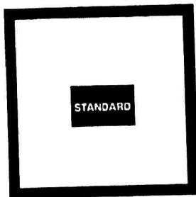
5. Press **STANDARD** and wait until the pH indicator stops flashing. The S2 indicator will begin flashing. The actual pH value will appear on the display and is based on the default or last calibration. Disregard the value.
