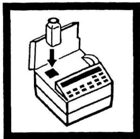
5. Add the contents of one SulfaVer 4 Reagent Powder Pillow to the sample cell (the prepared sample). Swirl to dissolve.
