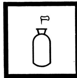
5. Remove the stopper and add the contents of one Sulfamic Acid Powder Pillow. Replace the stopper without trapping air in the bottle. Invert several times (the prepared sample).
