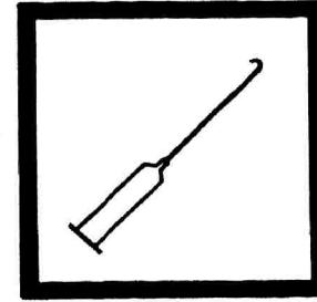
7. Insert a clean delivery tube into the Titration Cartridge. Attach the cartridge to the titrator body. See the Digital Titrator manual for assembly instructions.
