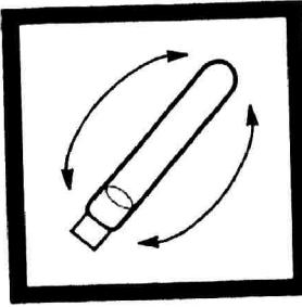
6. Hold the vial by the cap and over a sink. Invert gently several times to mix the contents. Place the vial in the preheated COD Reactor.
