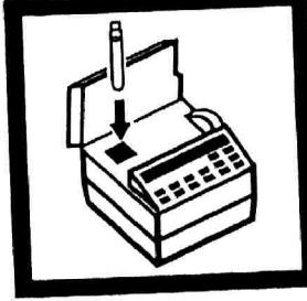
6. Place the blank into the adapter with the Hach logo facing the front of the instrument. Place the cover on the adapter.
