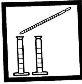
7. Pipet 1.0 mL of Nessler Reagent into each cylinder. Stopper. Invert several times to mix.
