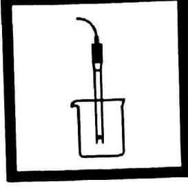
4. Place the electrode into a pH 4.01 buffer solution and press the Dispenser Button. The temperature will show the actual solution temperature if the temperature probe is connected.
