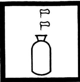
2. Add the contents of one Manganese Sulfate Powder Pillow and one Alkaline Iodide-Azide Reagent Powder Pillow.
