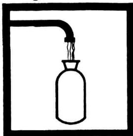
1. Collect a water sample in a clean, 300-mL glass-stoppered BOD bottle.
