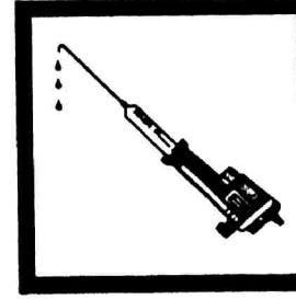
8. Hold the Digital Titrator with the cartridge tip pointing up. Turn the delivery knob to eject air and a few drops of titrant. Reset the counter to zero and wipe the tip.
