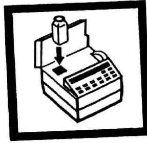
11. Place the prepared sample into the cell holder. Close the light shield.
