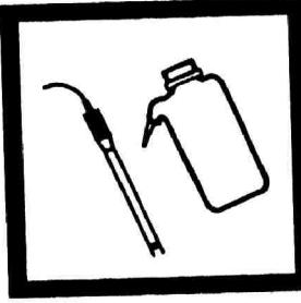
6. Rinse the electrode with deionized water and blot dry with a paper towel.
