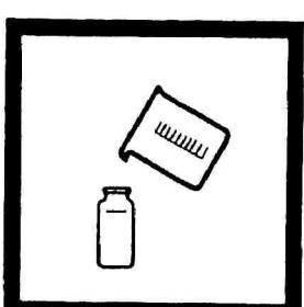
8. Fill another sample cell with 25 mL of sample (the blank).
